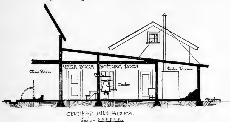
FIG. 94.—Elevation of certified milk house showing arrangement of milk spout through the wall from the weigh room into the milk room. There is no door connecting the two rooms.
