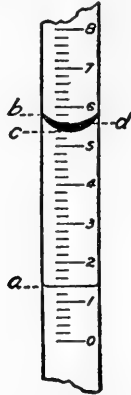
FIG. 111.—In milk testing the fat should be read from a to b , not to c nor to d , but in cream from a to b .
