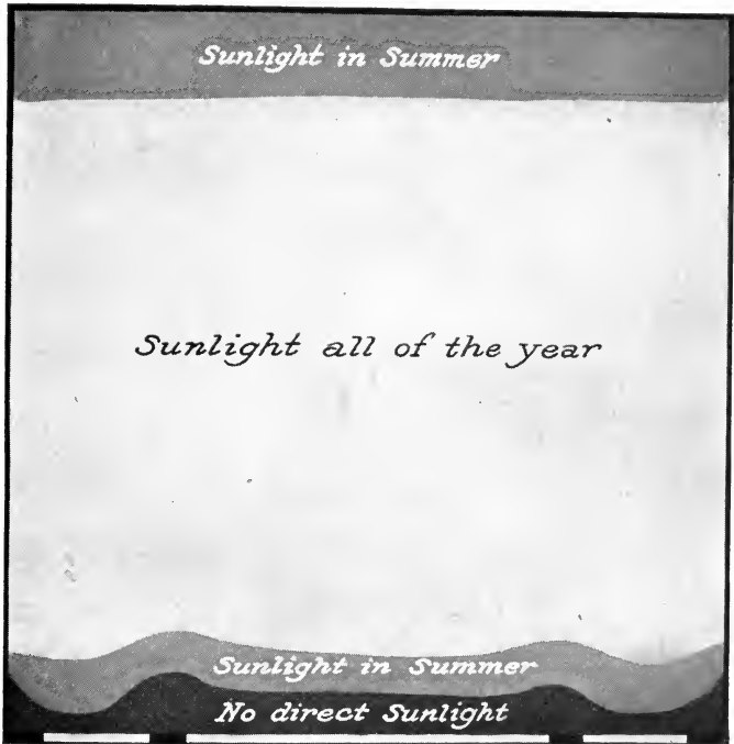
FIG. 66.—Floor of standard multiple-unit laying house, showing distribution of sunlight at different seasons, sun elevation at 10 o'clock.
