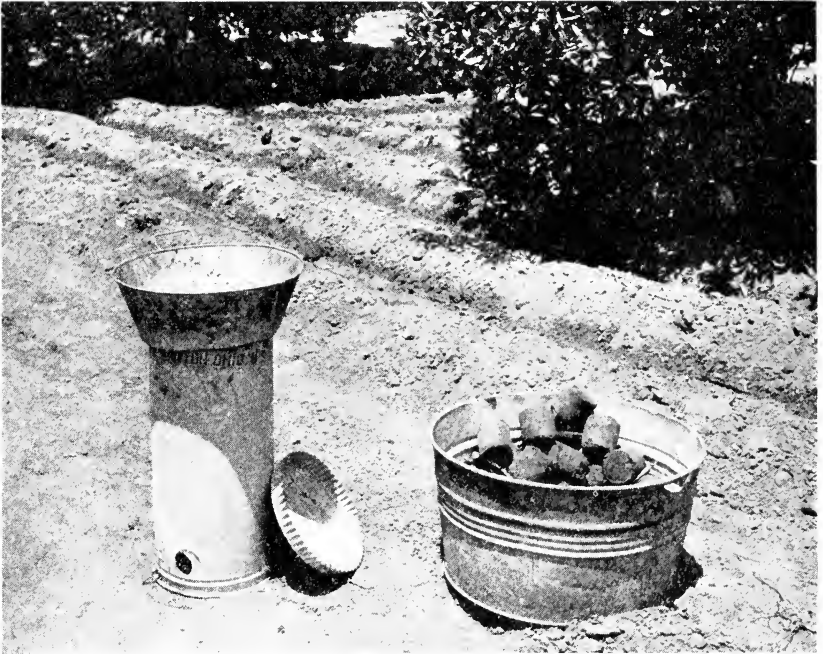
Fig. 11.—Briquette heater with funnel to facilitate filling, and tub for fuel storage. (From Bul. 398.)
