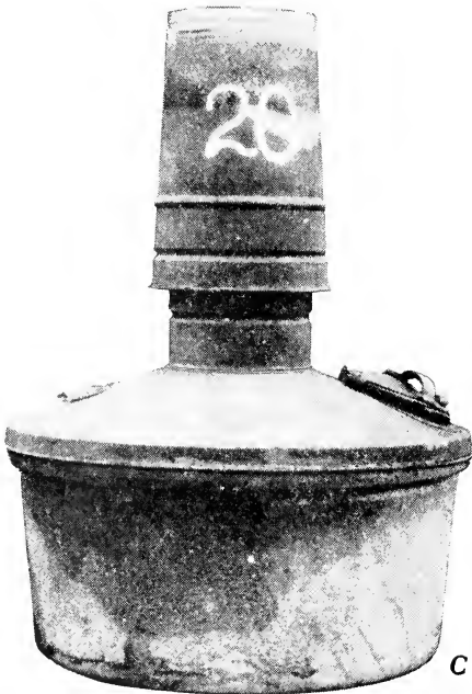
Fig. 5.—Early types of orchard heaters. A , National Baby Cone; B , National Exchange model, 5½-inch stack; C , National, double stack; and D , Hy-Lo double stack. These heaters are all of 9-gallon capacity; the illustrations are not of the same scale. (From Bul. 536.)
