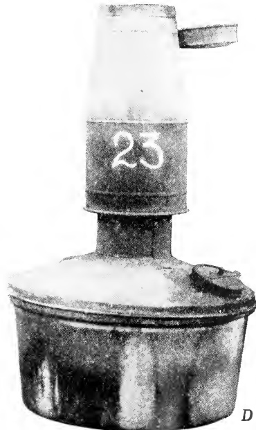
Fig. 5.—Early types of orchard heaters. A , National Baby Cone; B , National Exchange model, 5½-inch stack; C , National, double stack; and D , Hy-Lo double stack. These heaters are all of 9-gallon capacity; the illustrations are not of the same scale. (From Bul. 536.)
