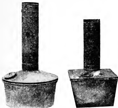
Fig. 6.—Round- and square-bowl orchard heaters of the “lazy-flame” type.
