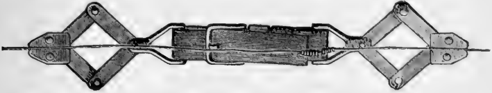
295. Parallel wire-stretchers in operation, the slack being pulled up by the strap.
