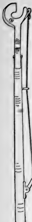
213. A good tool for heading-in out-stretching limbs and removing small stray branches.
