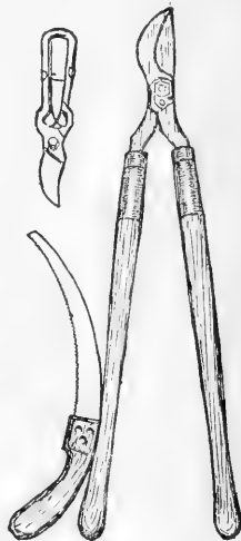
368. A set of good grape-pruning tools. Two-hand shears, one-hand shears, curved saw.
