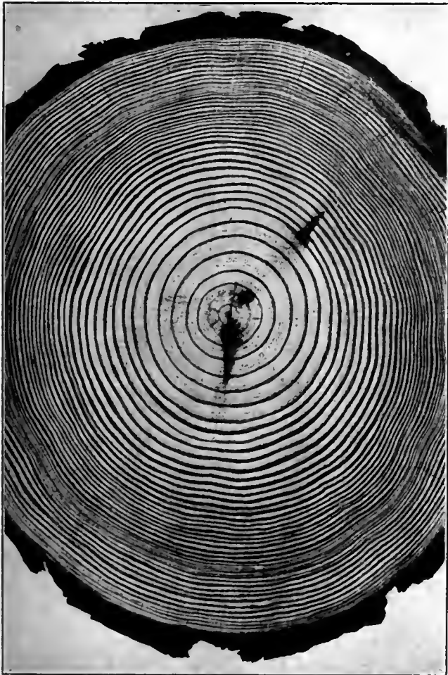
THE GROSS CHARACTER OF THE SHORTLEAF PINE IN CROSS-SECTION
