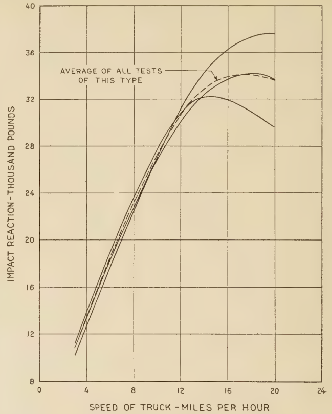
FIG. 12.—MOTOR-TRUCK IMPACTS ON A 6-INCH 1:2:4 CONCRETE
