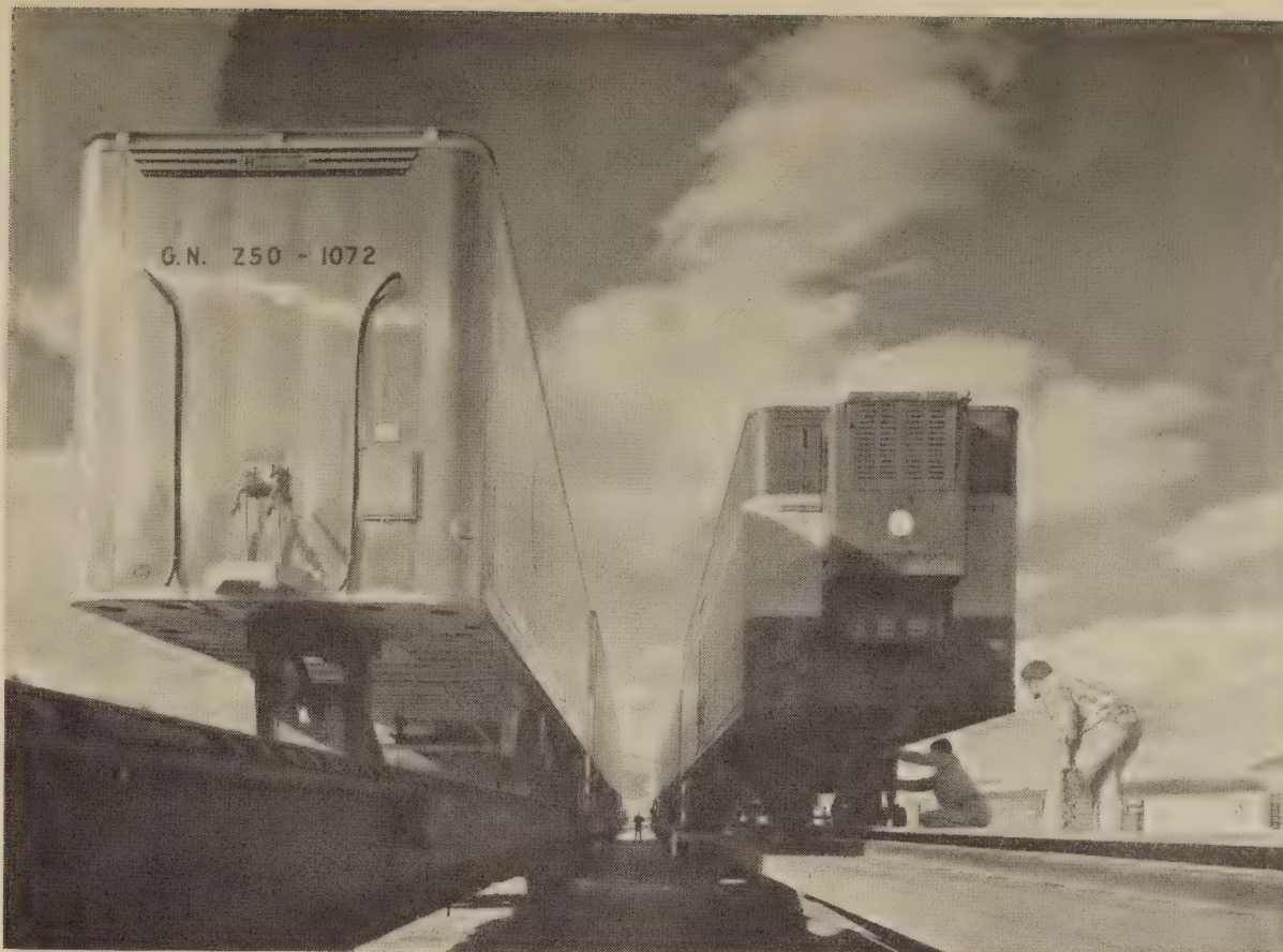
When highway trailers are hauled on rail flatcars in piggyback operations, highway transportation is an essential part of the overall service.
