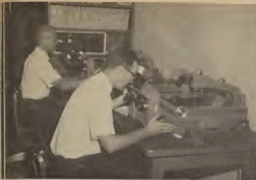
Two of the photogrammetric instruments, point transfer device (left) and stereocomparator (below), that were used in the evaluation presented in this article. The point transfer device was used to drill pass points on photographic plates; the stereocomparator was used to measure photogrammetric x and y plate coordinates.
