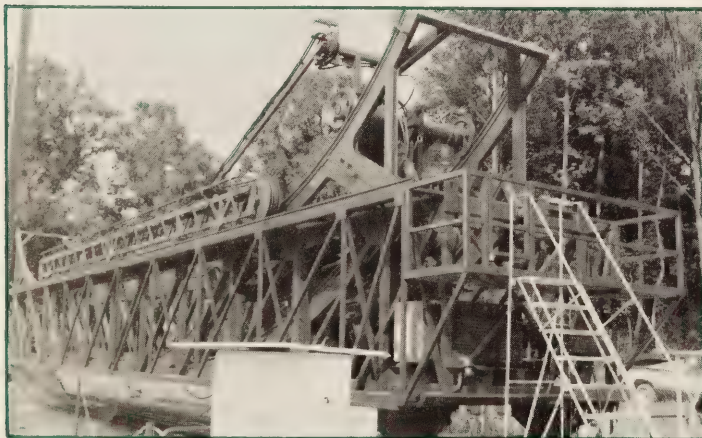
The ALF, part of the Pavement Testing Facility at the Turner-Fairbank Highway Research Center in McLean, Virginia, simulates truck traffic on a full-scale pavement.
