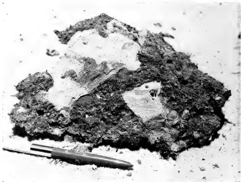
Figure 6. A block of the "breccia" shown in Figure 5. The white fragments of limestone are embedded in a matrix consisting of abundant pebbles and grains of phosphate, quartz sand and clay.
