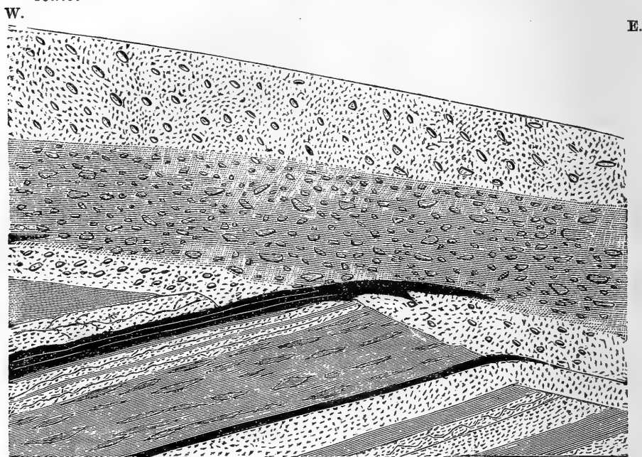
Fig. 8.—Section showing Coal-seams squeezed into drift during the deposition of the lowest gravel on Hirwain Common.—Natural scale.
