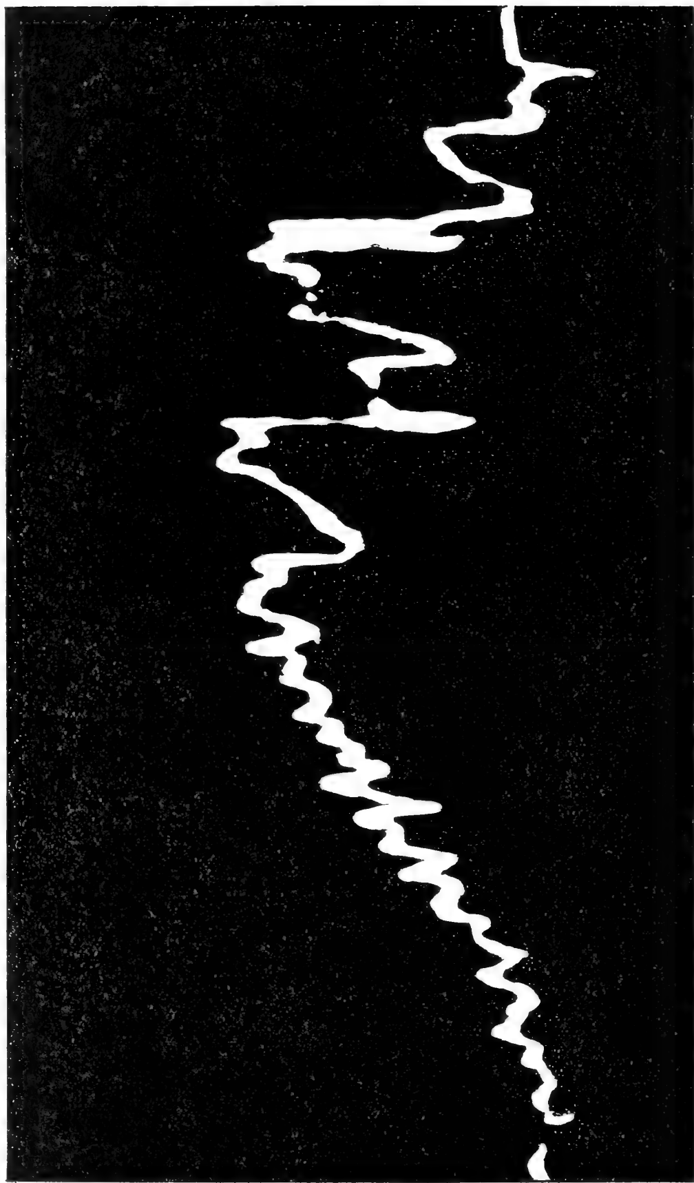
Fig. 1.—The record of the earthquake of March 24th, 1903, registered at Birmingham by an Omori horizontal pendulum.
