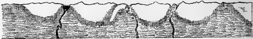
Fig. 2.— Mode of occurrence of alabaster pillars at Chellaston. (Length of section = 90 feet.)
