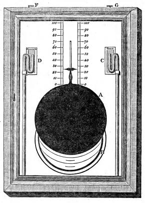
"The black disc A is a thin plate of metal attached to a rod coming up from the valve behind the index frame, in which there is a slit for the pin which carries the index to pass." The portion of the circle B, which is uncovered by the disc, represents the aperture, or gas-way into the main pipe. D is a pressure gauge connected with the main on the gasometer side
