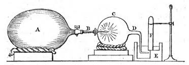
A. The bladder and stopcock containing the mixed gases. B. The thermometer tube cemented into the stopcock, and passing through the cork of the globe. C. A globe, to the mouth of which a cork was fitted. The cork being slipped upon the tube, the stream of mixed gases was fired, and the tube and cork then introduced to the globe. D. The quill going from the globe to the mercurial trough. E. The trough. F. A gas jar to receive the elastic fluid evolved.
