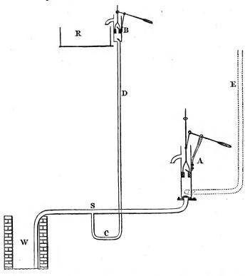
A is a pump which draws water from the well W, about twelve feet deep. CD is a pipe which branches from the ingress pipe S, and ascends fifteen feet above S to supply (by means of a second pump B) the reservoir R. The bend in the pipe at C was made that it may conform to the floor of an underground cellar.
