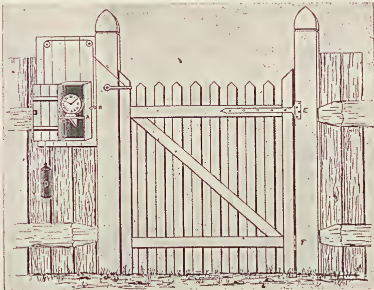
A. Clock case. B. Lever releasing weight. C. Cord attached to hasp of gate. D. Weight. E. Ordinary hinge. F. Crank hinge.
