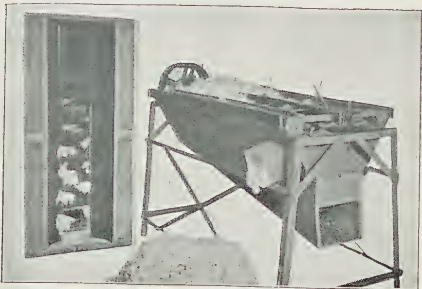
PLATE 6.—THE LIENAU KAPOK-CLEANING MACHINE. INTERIOR
