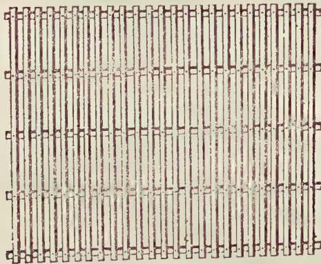
FIG. 2a.—Lattice-work transfer tray (original).
