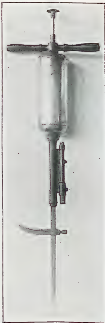
PLATE 51.—“VERMOREL EXCELSIOR” HAND-INJECTOR, FOR FUMIGATING CANE LAND WITH BISULPHIDE OF CARBON (LENGTH 44 IN., WEIGHT ABOUT 14 LB.)
