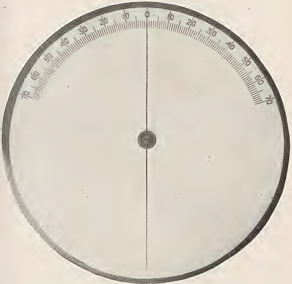
PLATE 55.—DIAL OF AUTOMATIC WATER FINDER, SHOWING MAGNETIC NEEDLE AT ZERO.
