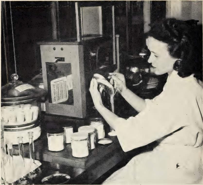
FIGURE 7.—An inspector carefully transfers a sample of sugar, which she has weighed on an analytical balance, to a flask in preparation for a polarization test that will determine the purity of the sugar.
