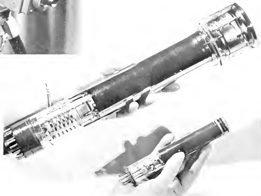
LEFT: INTERIOR OF SMALL CAMERA SHOWING THE VIDICON TUBE AT THE LOWER RIGHT CORNER OF THE CASE. BELOW: A COMPARISON OF THE RELATIVE SIZES OF THE STANDARD IMAGE ORTHICON CAMERA TUBE AND THE NEWLY DEVELOPED VIDICON.
