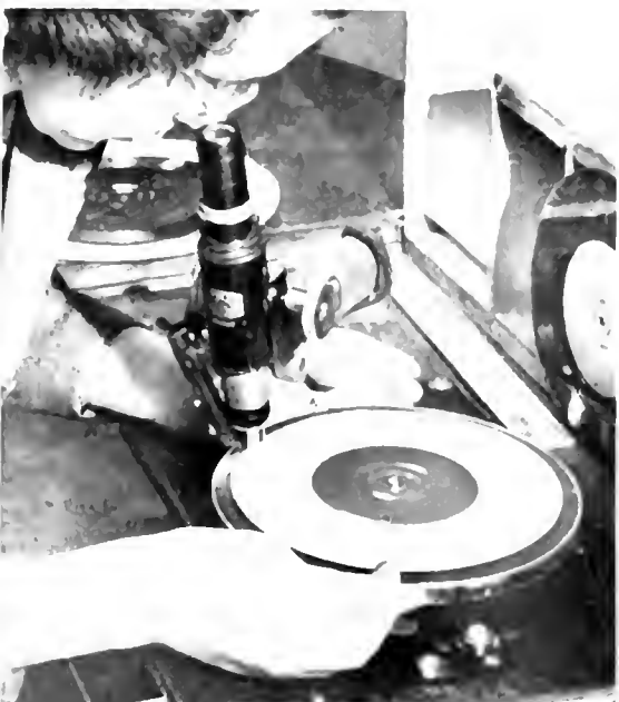
Exact centering of a 45-rpm record is assured by checking the movement of the outer rim under a microscope.
