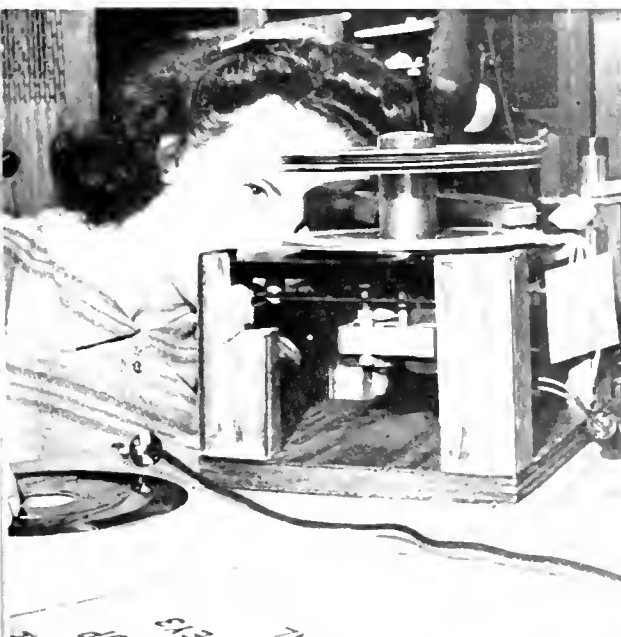
An inspector checks the operation of the disc-changing cycle of a record player.
