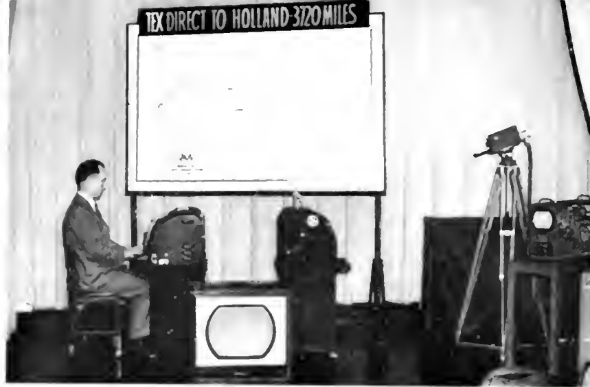
AT THE FIRST PUBLIC DEMONSTRATION OF TEX, THE AUDIENCE GETS A CLOSE-UP VIEW OF THE TELEPRINTER COPY ON A TELEVISION SCREEN SUPPLIED WITH SIGNALS PICKED UP BY THE VIDICON CAMERA AT RIGHT.
