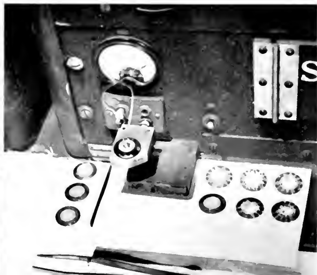
INK PLACED ON VIBRATING CRYSTALS FORMS INTO PATTERNS WHICH INDICATE THE ACCURACY OF MANUFACTURE.
