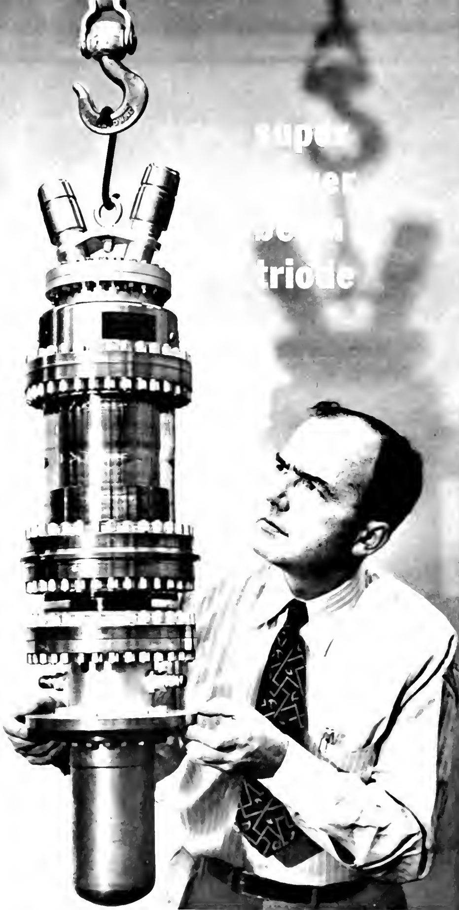
DR. I. P. GARNER OF THE LANCASTER, PA., PLANT EXAMINES ONE OF THE REMARKABLE 500-KILOWATT TUBES WHICH HE AND HIS ASSOCIATES DEVELOPED.
