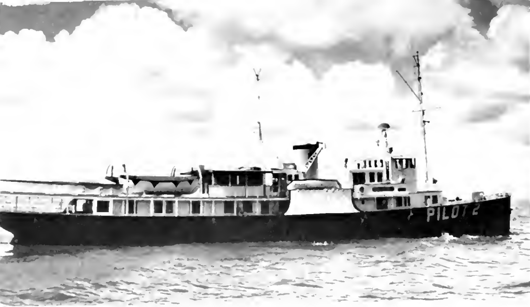
PILOT BOAT NEW JERSEY, SHOWING THE UNUSUAL "HALO" ANTENNA AMIDSHIPS WHICH PICKS UP TELEVISION SIGNALS FROM NEW YORK AND PHILADELPHIA REGARDLESS OF THE POSITION OF THE SHIP WHEN STATIONED OFF NEW YORK HARBOR.
