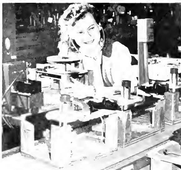
Record players undergo a listening test, one of the final steps in the manufacture of the high-fidelity instruments.
