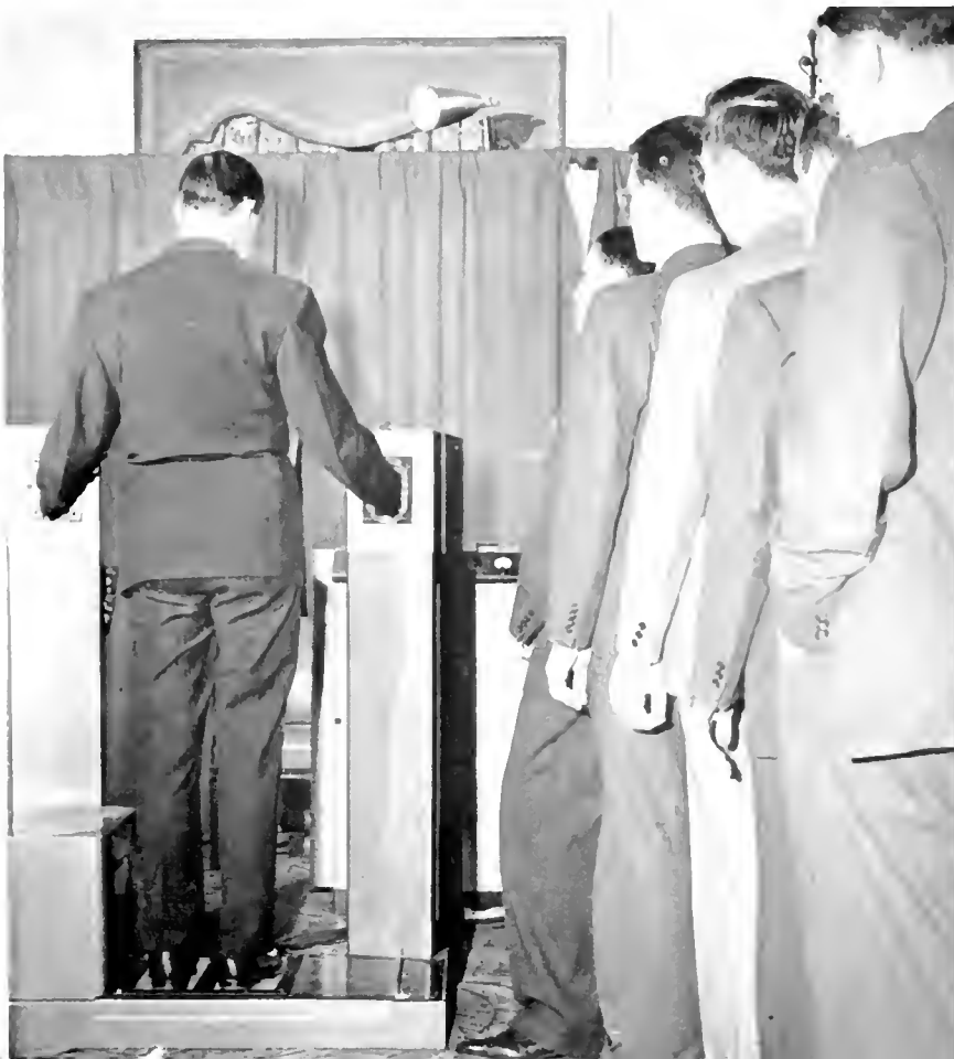
SAFETY OF WORKERS IN RADIOACTIVE MATERIALS IS ASSURED BY THE USE OF THIS MONITOR, DEVELOPED BY RCA. THE DEVICE INDICATES BY COLORED LAMPS THE PRESENCE AND INTENSITY OF DANGEROUS CONTAMINATIONS ON HAND AND FEET.
