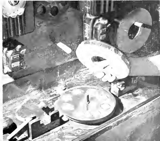
GROUPS OF WAFERS ARE POCKETED IN A FLAT PLATE AND LOPPED TO EXACT DIMENSIONS BY APPLYING ABRASIVE MIXTURES.
