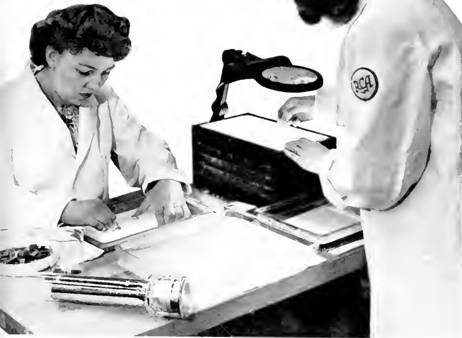
EXCESS METAL IS ERASED FROM THE MASTER (LEFT) AS ANOTHER WORKER EXAMINES A SCREEN FOR FLAWS.
