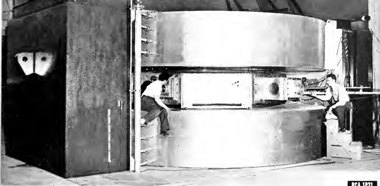
THE 130-INCH CYCLOTRON INSTALLED AT THE UNIVERSITY OF ROCHESTER USES THE ULTRA-SENSITIVE RCA MULTIPLIER PHOTOTUBE (RIGHT) TO MEASURE THE RADIATIONS PRODUCED WITHIN THE HUGE DEVICE.
