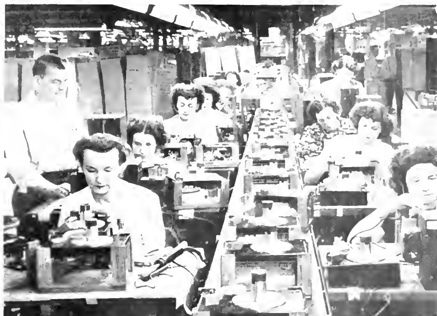
A moving conveyor separates the assembly group on the left from testers and inspectors of the finished product on the right.
