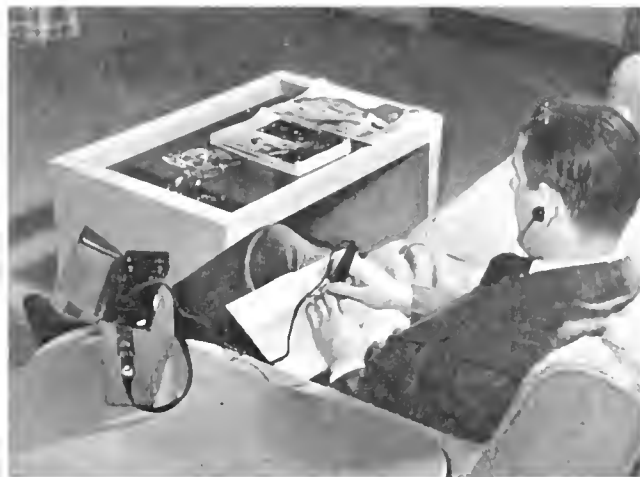
BELOW: THIS MODEL OF ELECTRONIC READING AID CONVERTS LETTERS INTO THEIR SPOKEN SOUNDS. AT RIGHT: EARLIER MODEL OF READING AID PERMITS USER TO RECOGNIZE LETTERS BY DISTINGUISHING SOUNDS WHEN SCANNED BY ELECTRON BEAM IN HAND-HELD STYLUS.
