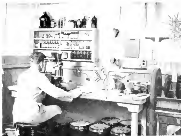
IN THIS CONTROL LABORATORY GLUES AND LACQUERS ARE CHECKED FOR THEIR RESISTANCE TO TROPICAL CONDITIONS.
