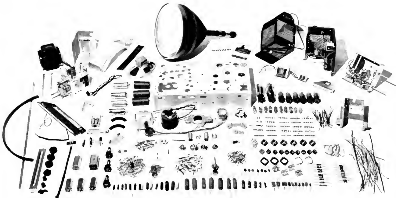
SOME OF THE HUNDREDS OF PARTS AND SUB-ASSEMBLIES THAT GO INTO THE MAKING OF A 12 \frac{1}{2} -INCH TELEVISION RECEIVER.
