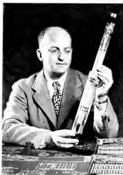
A NEW TUBE, CALLED THE GRAPHECHON, CAN STORE FOR MORE THAN A MINUTE CERTAIN TYPES OF ELECTRICAL SIGNALS WHICH ORDINARILY WOULD FADE OUT IN A MILLIONTH OF A SECOND WHEN TRACED ON A FLUORESCENT SCREEN.
