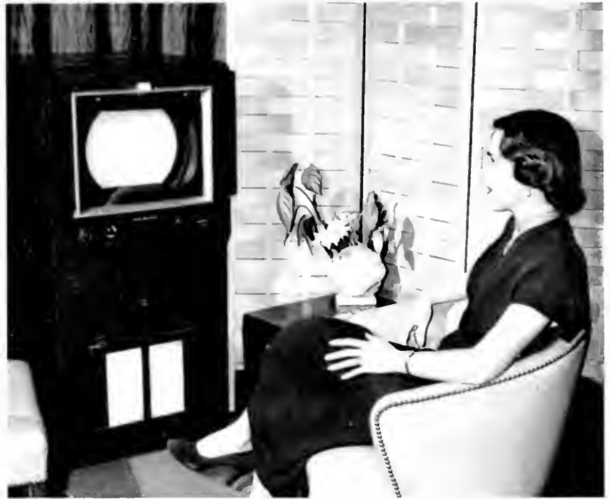
DEMONSTRATION MODEL OF TELEVISION RECEIVER EMBODYING RCA'S ALL-ELECTRONIC COLOR SYSTEM AND RCA TRI-COLOR DIRECT-VIEW KINESCOPE TUBE.
