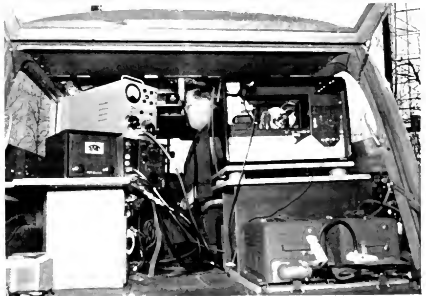
EXTERIOR AND INTERIOR VIEWS OF THE STATION WAGON WHICH IS BEING USED THROUGHOUT THE NORMAL SERVICE AREA OF THE BRIDGEPORT UHF "SATELLITE" TO MEASURE THE STRENGTH OF THE TRANSMITTED SIGNALS AT DIFFERENT DISTANCES FROM SUCCESS HILL.
