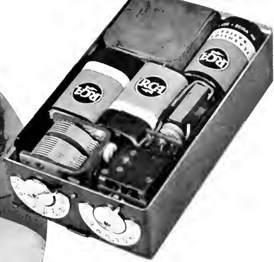
CONTAINING FOUR MINIATURE TUBES AND ALL BATTERIES, THE RECEIVER IS SMALL ENOUGH TO FIT EASILY INTO A POCKET OR MILADY'S HANDBAG. BELOW: COMPARISON OF PREVIOUS "PERSONAL" RADIO AND THE LATEST MODEL.
