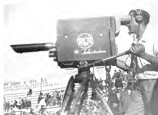
USING A TELEPHOTO LENS, A TELEVISION CAMERAMAN FOCUSES ON ACTION IN A FAR CORNER OF A SPORTS ARENA.
