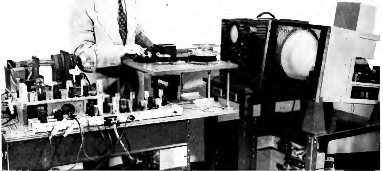
PRINCIPAL ELEMENTS OF THE SENDING TERMINAL OF RCA ULTRAFAX. THE CATHODE RAY TUBE (LEFT) GENERATES THE "FLYING SPOT" OF LIGHT FOR SCANNING MESSAGES ON A FILM STRIP AS IT PASSES THROUGH THE UNIT ON THE CENTER TABLE. MONITORING APPARATUS IS AT THE RIGHT.
