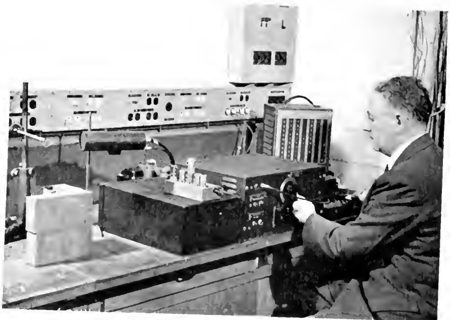
DR. G. A. MORTON OF RCA LABORATORIES SEATED BEFORE AN EXPERIMENTAL MODEL OF SCINTILLATION COUNTER EMBODYING A NEWLY DEVELOPED RCA MULTIPLIER PHOTOTUBE.
