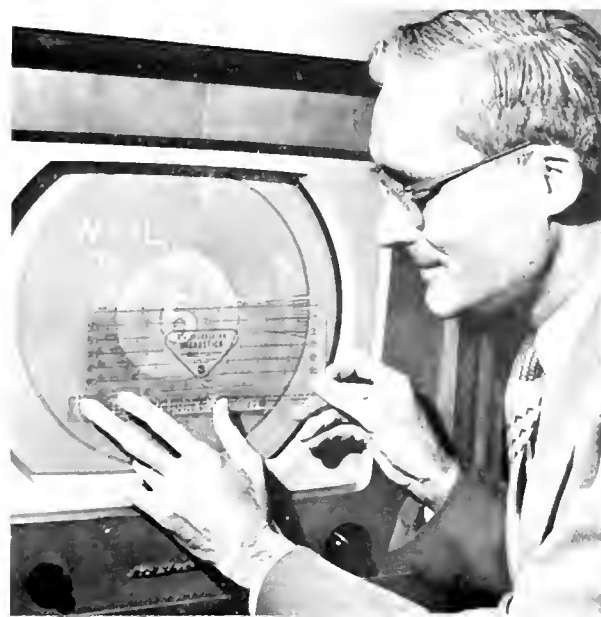
JOHN MEAGHER OF THE RCA TUBE DEPARTMENT, DEMONSTRATES THE "MICROSTICK", A TRANSPARENT PLASTIC RULER WHICH HE DEVELOPED TO SIMPLIFY TELEVISION PICTURE ANALYSIS.
