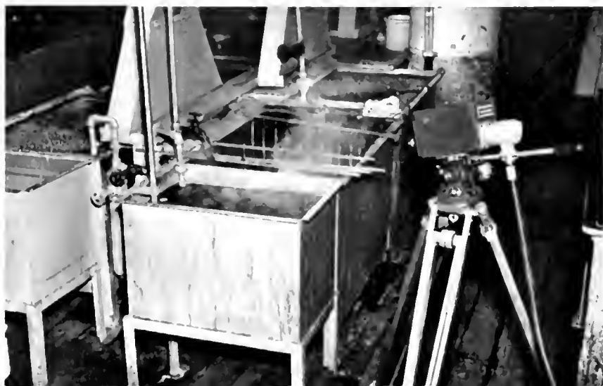
THE RCA INDUSTRIAL TELEVISION SYSTEM IS EXPECTED TO FIND WIDE ACCEPTANCE IN THE REMOTE-OBSERVATION OF MANUFACTURING PROCESSES. HERE A VIEW OF A CHEMICAL OPERATION IS TRANSMITTED BY THE VIDICON CAMERA TO A SCREEN SOME DISTANCE AWAY.
