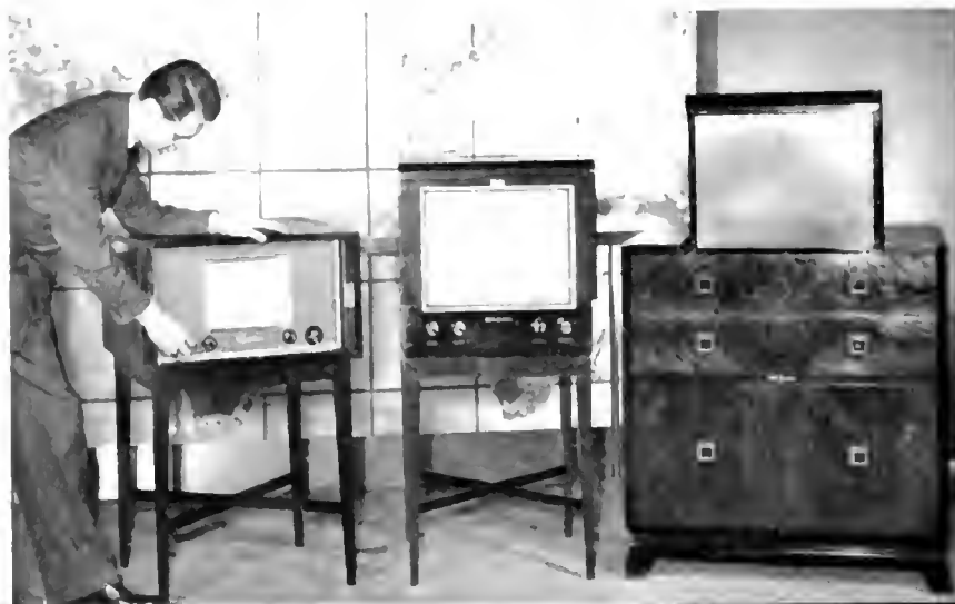
STANDARD RCA VICTOR TELEVISION RECEIVERS — LEFT TO RIGHT: TABLE MODEL WITH A 10-INCH GLASS TUBE; TABLE MODEL WITH A 16-INCH METAL-CONE TUBE, AND A PROJECTION-TYPE CONSOLE.
