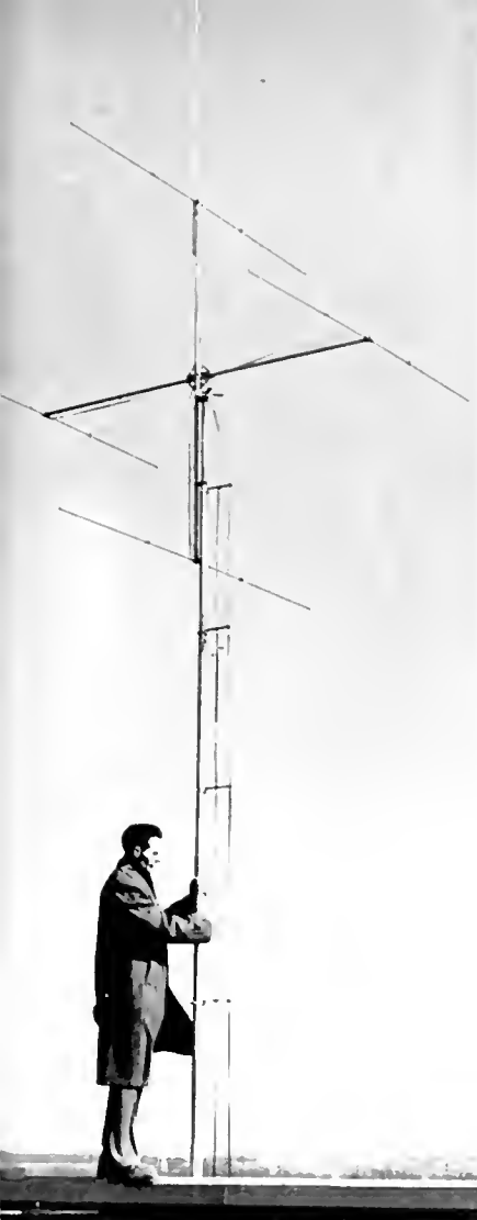
O. M. WOODWARD OF RCA LABORATORIES STAFF MAKES ADJUSTMENT ON COMBINATION HIGH- AND LOW-BAND TELEVISION ANTENNA WHICH HE DEVELOPED.
