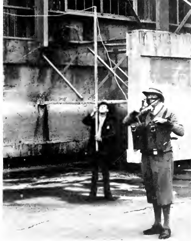
THIS EARLY VERSION OF THE PORTABLE TRANSMITTER WAS LARGE AND CUMBERSOME AND REQUIRED A LENGTH OF WIRE FOR ITS ANTENNA.
