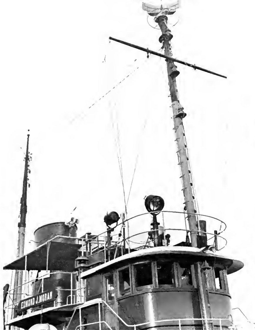
LEFT: RADAR ANTENNA OF THE "MORAN" IS LOCATED AT PEAK OF FOREMAST.
