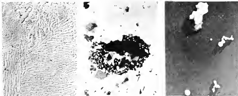
THREE TYPICAL EXAMPLES OF ELECTRON MICROSCOPY MADE POSSIBLE BY THE RCA ELECTRON MICROSCOPE. LEFT TO RIGHT: FORMATION OF PEARLITE IN STEEL; SAMPLE OF FACE POWDER MAGNIFIED 15,000 TIMES, AND DUST PARTICLES WHICH CAST THEIR SUBMICROSCOPIC SHADOWS AFTER AN ENLARGEMENT OF 24,000 TIMES.
