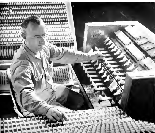
At the "Lumi-Tron" lighting board, 2,000 lighting controls are within reach of the technician.
