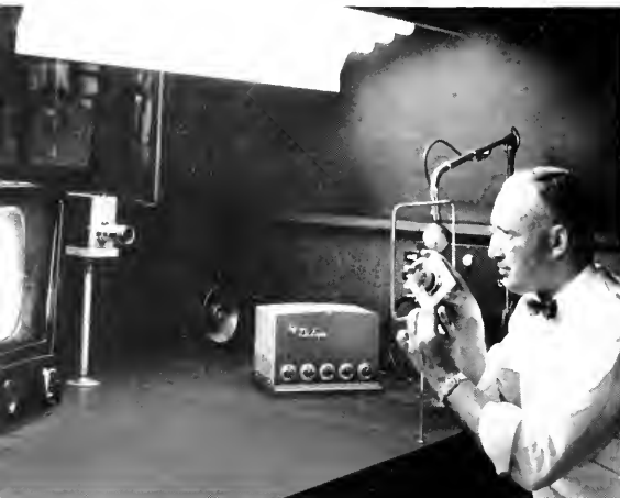
At the Bulova Watch Company in Providence, R. I., "TV Eye" permits visual communication between engineers, left, and production section, right, in separate buildings.
