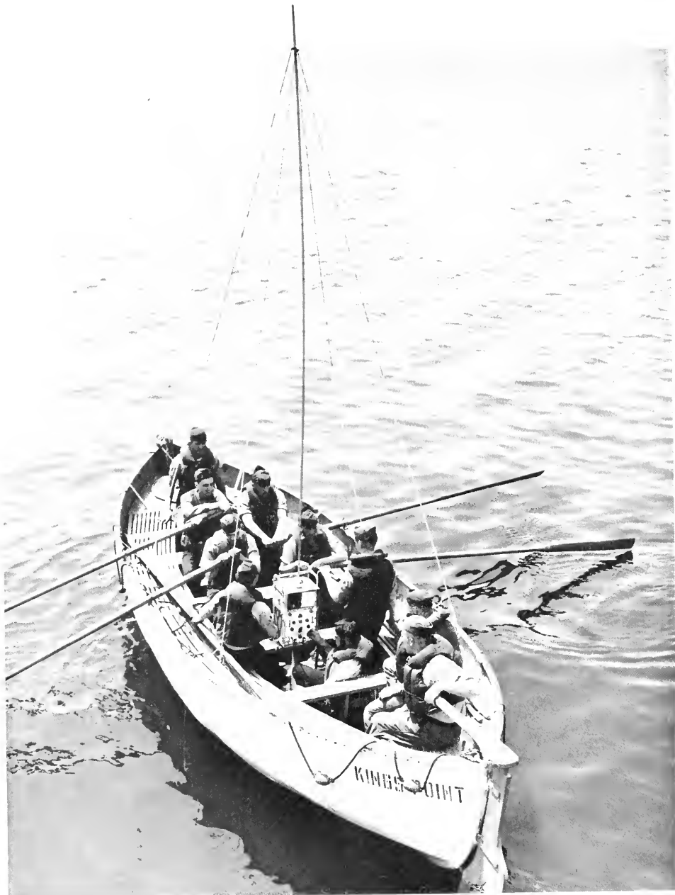
Radiomarine's new portable lifeboat radio is demonstrated by cadets of the U. S. Merchant Marine Academy, Kings Point, N. Y. Two cadets in the center are cranking the 60-pound emergency send-receive unit which is topped by a 15-foot antenna mast. (Story on page 18)
