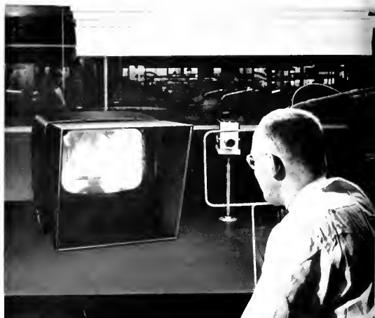
At the Bulova Watch Company in Providence, R. I., "TV Eye" permits visual communication between engineers, left, and production section, right, in separate buildings.
