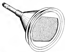
DOT-SCREEN TUBE FOR COLOR TV Spontaneous Emission
