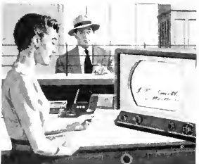
RCA vidicon camera in a bank, lets tellers verify the signatures on checks by television.
