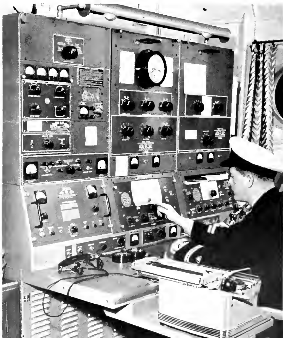
In the radio room of the icebreaker d'Iberville , Radio Officer Charlie Seaman tunes in one of the several RCA radiotelegraph units built into the console.
