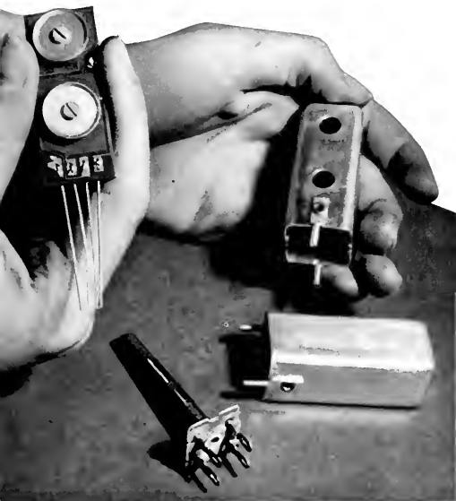
A complete printed circuit i.f. transformer and its shield (in hands) are compared with older type components (on table) to show comparative sizes.
