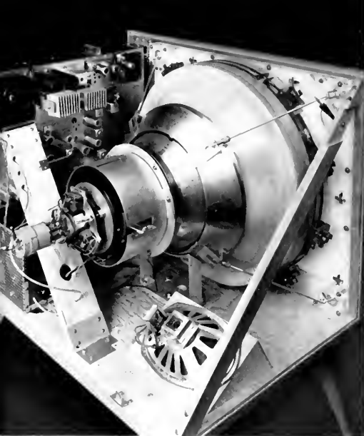
Rear view of the new RCA 21-inch simplified color TV set shows how circuitry has been reduced.
