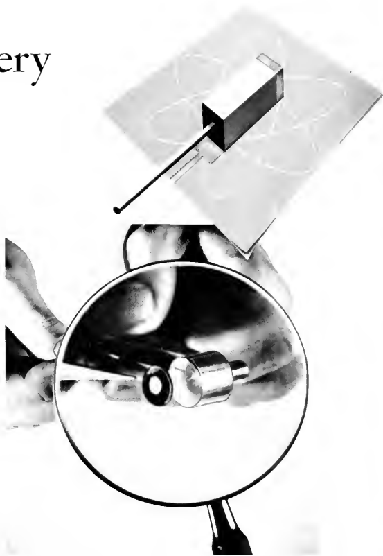
Both elements of the battery — semi-conducting crystal, held in tweezers, and layer of radioactive material, on cylinder — are shown under magnifying glass.
