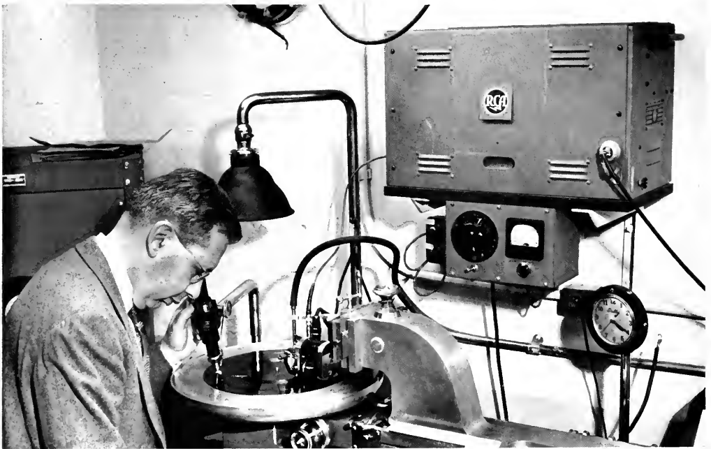
The author examines a master recording produced by the advanced "New Orthophonic" techniques developed by RCA Victor engineers. The cutting stylus is electronically heated to give a wide frequency range throughout the length of the groove.
