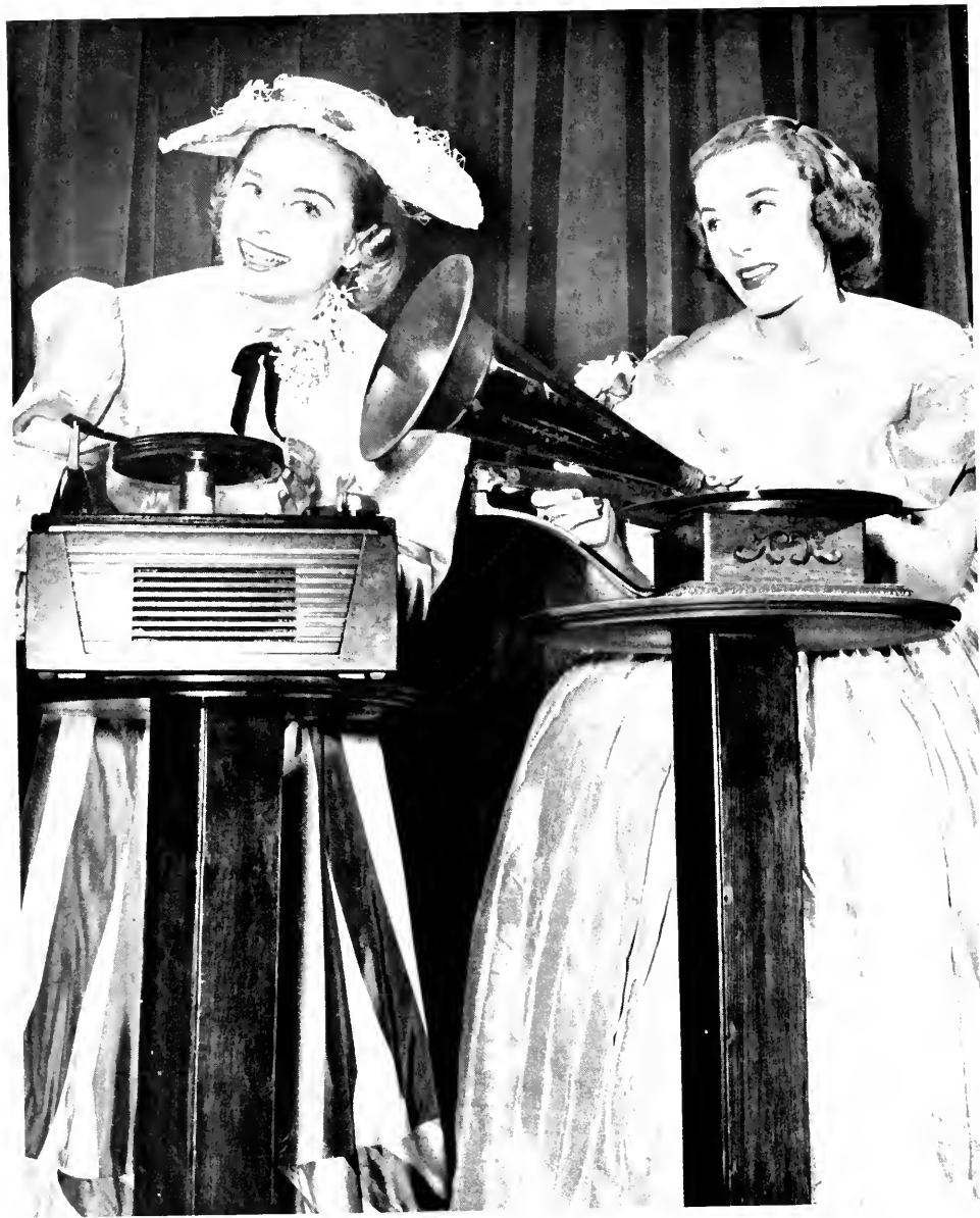
The phonograph record players span more than fifty years of progress. (Left): the latest RCA Victor 3-speed "Victrola" phonograph; (right) and early spring-wound record player.
