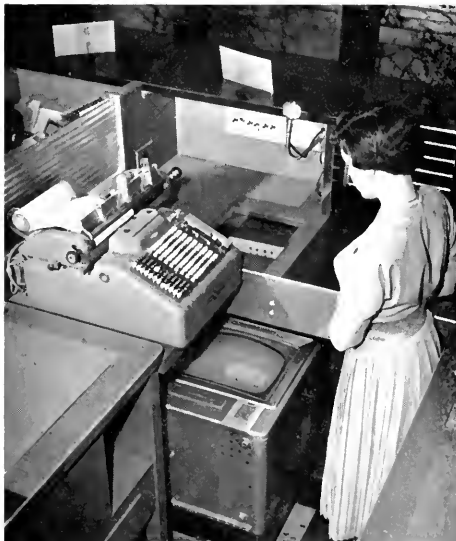
Largest installation yet of "TV Eye" helps to speed banking operations at the Provident Institution for Savings in Boston. File clerk, above, holds signature cord before the camera for viewing by teller, right.
