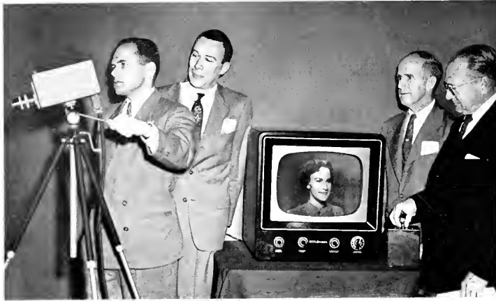
Dr. V. K. Zworykin, (right) Vice President and Technical Consultant, RCA Laboratories Division, and staff members, demonstrate simplified closed-circuit television system for the home, using Vidicon camera attached to standard home receiver. Others, left to right, are G. W. Gray, W. S. Pike and L. E. Flory.
