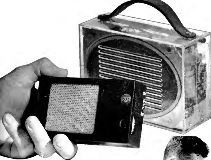
Transistorized broadcast radio receiver capable of fitting into a breast pocket is shown in comparison with an earlier model equipped with a 4 x 6-inch speaker.
