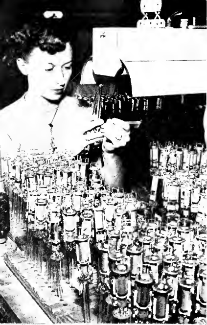
An inspector examines the assembly of an electron gun, to assure that this fundamental element of a television picture tube conforms to rigid specifications.
