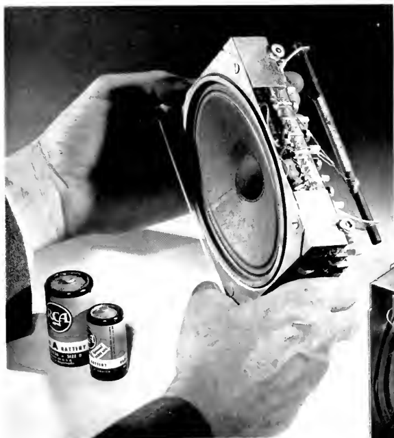
Front (left) and rear views of the experimental completely transistorized radio receiver developed at RCA Laboratories. The row of transistors is pointed out below.
