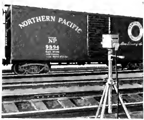
In a railroad yard, RCA vidicon camera lets employees check car numbers at long range.
