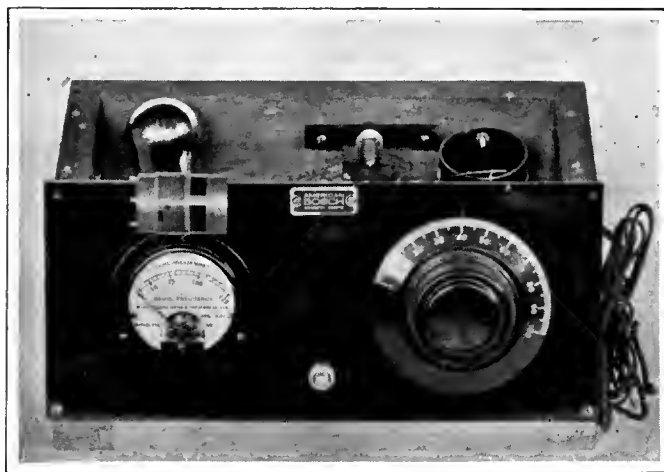
THE R.F. OSCILLATOR USED BY BOSCH TO MATCH COILS
