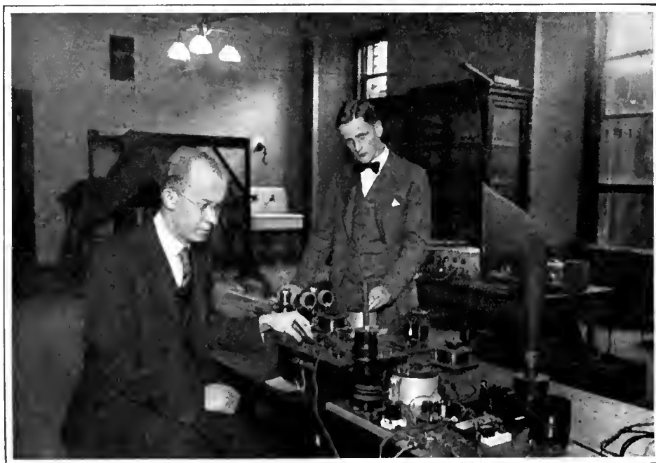
A CORNER OF ONE OF THE COLUMBIA UNIVERSITY LABORATORIES Making measurements on a resistance-coupled audio amplifier in the Hartley Laboratory
