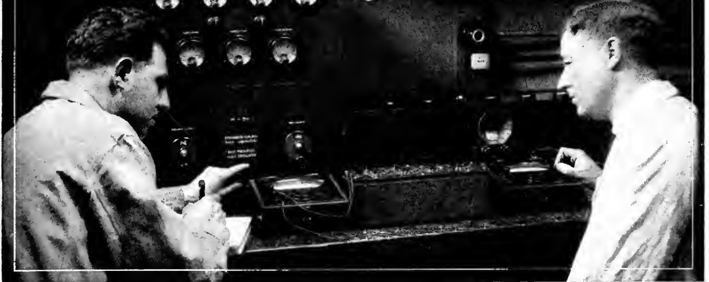
Stromberg-Carlson engineers testing the audio-frequency characteristics of one of their No. 744 receivers. The apparatus consists of a "beat frequency" oscillator which produces the audio tones, and meters for measuring the extent to which these frequencies are amplified within the receiver
