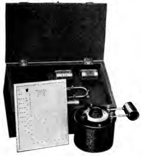
THE GENERAL RADIO WAVEMETER The wavemeter has coils to cover all the amateur wave bands. The small U-shaped coil in the box is for the 5-meter band
