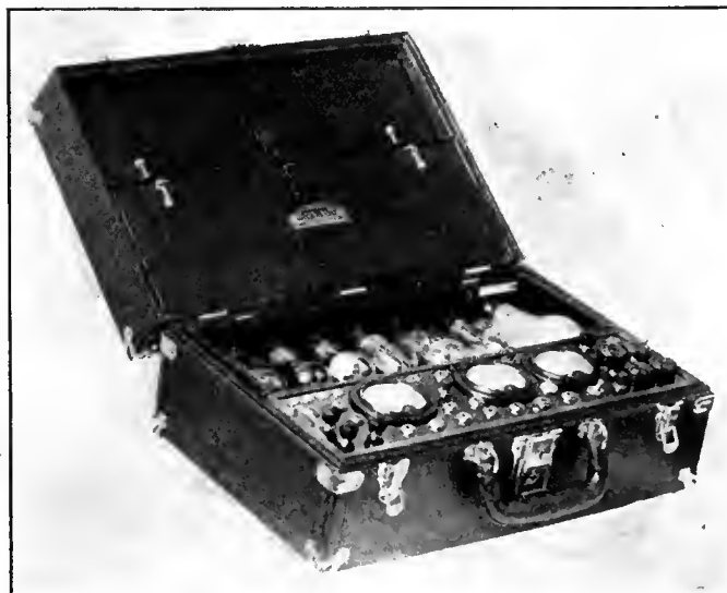
In general service work the Diagonometer is carried in a compact leather case of the type shown above. The case also provides space for accessories and tubes.
