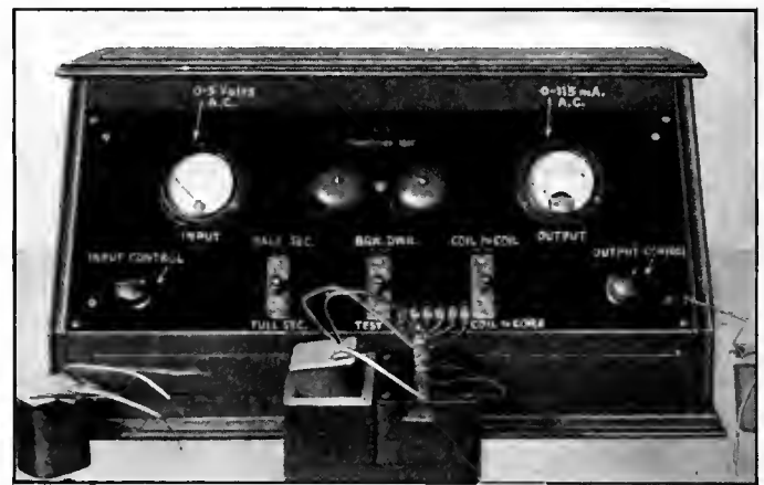
The output transformer test set.
