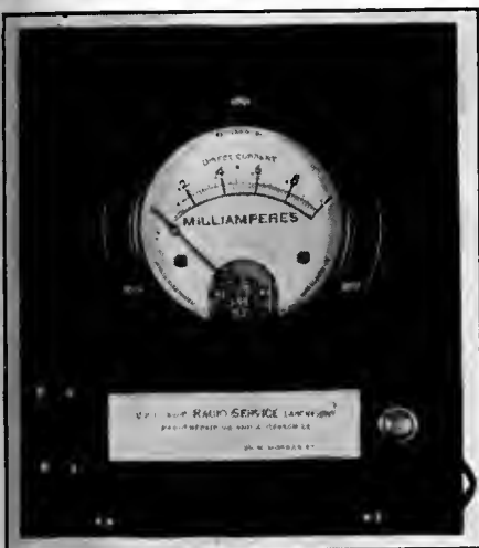
Front view of output meter.
