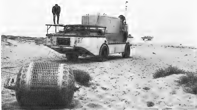
Figure 7. Field operations at Surf, California, June 1967. In foreground are mobile detector vehicle ("ball") and LARC-V with instrument shelter. In background is DUKW vehicle used in support of operations.
