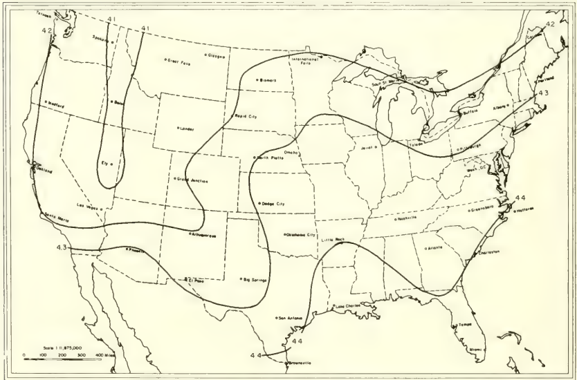
FIGURE 7.17. August values of 300-mi propagation path absorption loss (in dB) to be exceeded 1 percent of the time for a frequency of 10,000 Mc/s.
