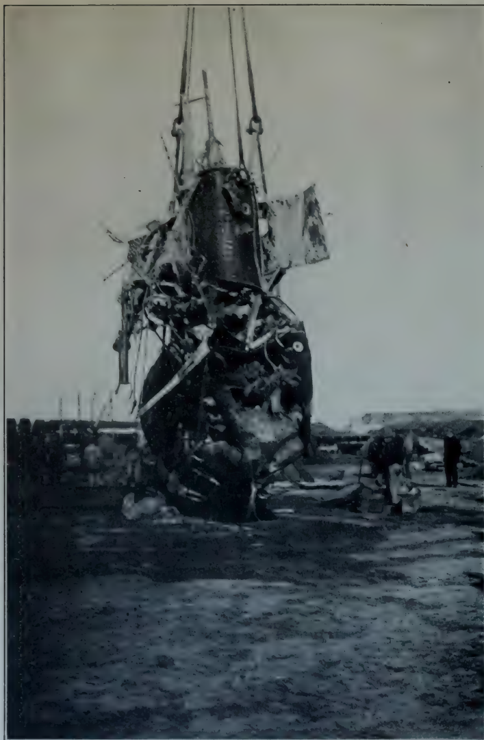
The effect of a mine on a submarine. In all, 178 raiders of the deep lie somewhere on the floor of the ocean.
