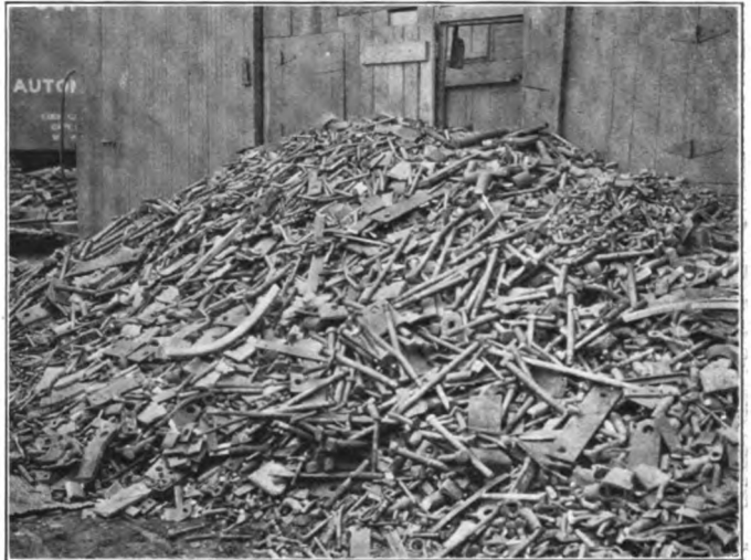
Fig. 2—Wrought Iron Scrap Ready to Be Made Into Piles for the Rolling Mill
