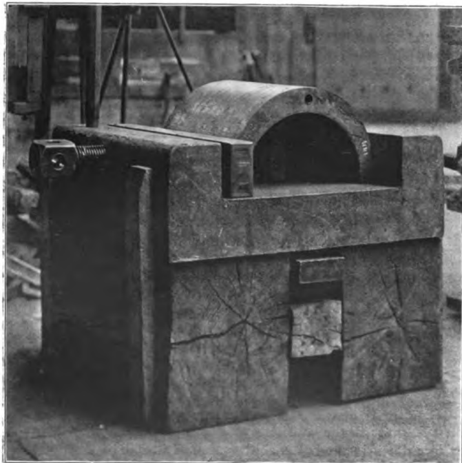
The Type of Hand Press Used for Closing Crown Brasses
