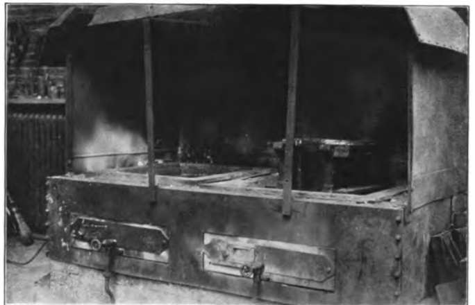
Babbitt Furnace, Showing Driving Box in Place for Removal of Hub Liner
