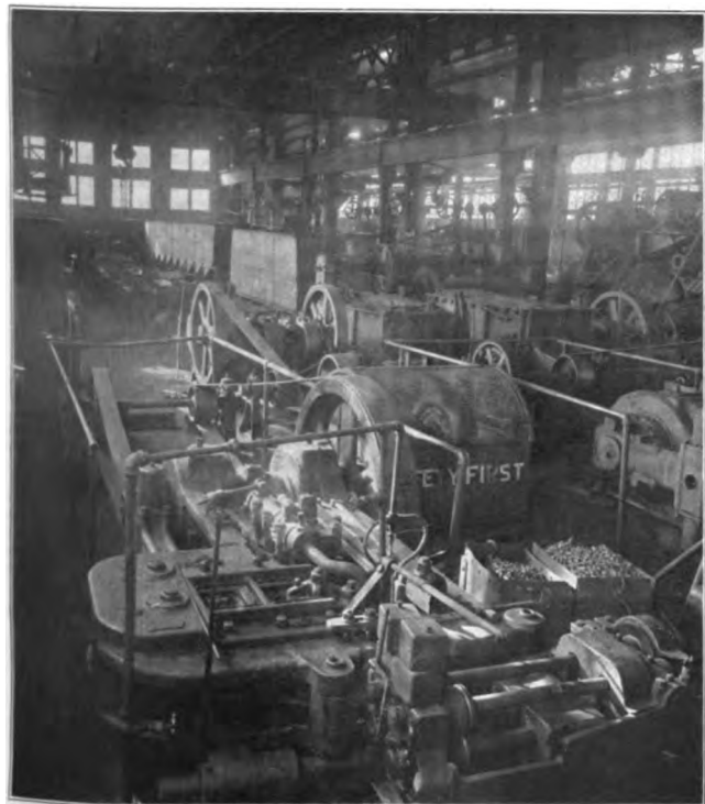
Rivet Heading Machine with Overhead Crane and Storage Bins in the Background
