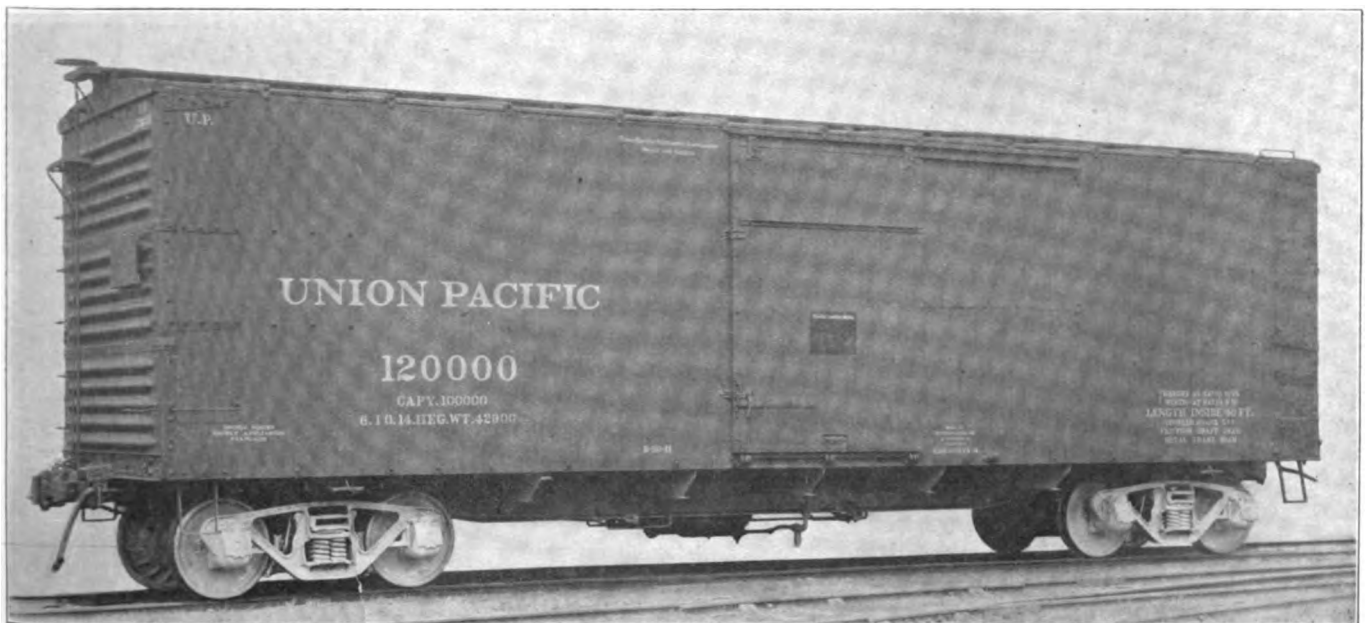
Steel Underframe Box Car for the Union Pacific
