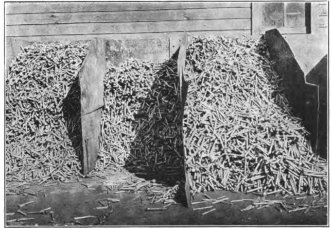
Fig. 8—Carriage Bolts Made on Automatic Bolt Machines
