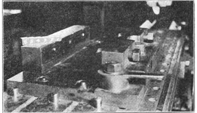
Fig. 8—Shoe and Wedge Planer Chuck
