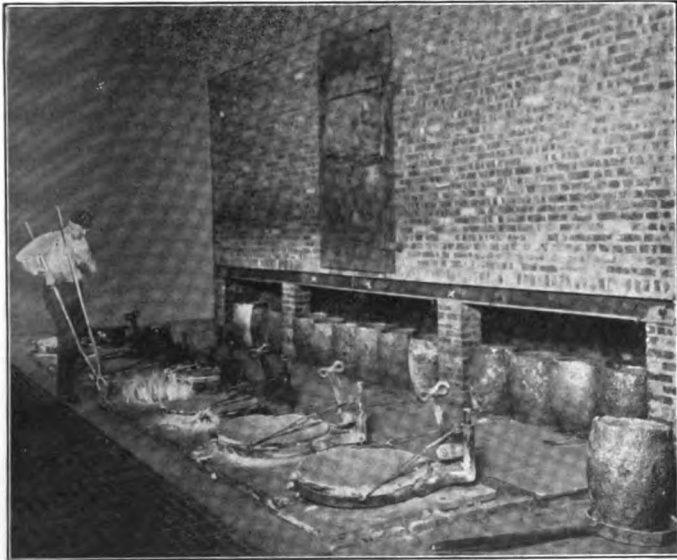
Pit Furnaces Operated with Oil and Gas.
