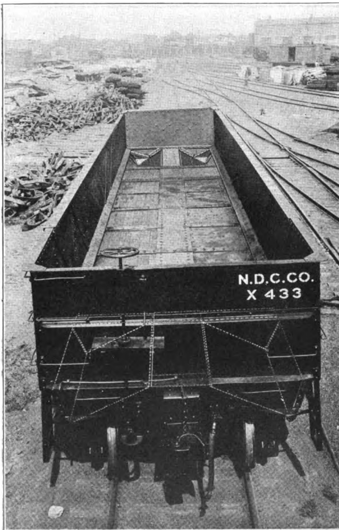
The Hartend Car Showing the Side Hoppers at the Ends
