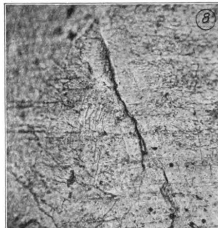
Fig. 3—Oxy-acetylene weld showing heavy slipping at grain boundary. This is not a crack, but shows a weakness.
