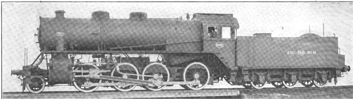
Consolidation Type Locomotive for Belgium Built in Record Time
