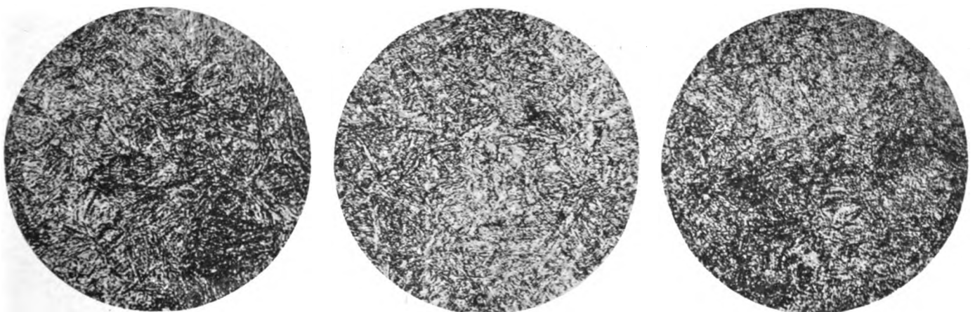
Fig. 1. Microphotographs of Chrome Molybdenum Steel Showing Similarity of Microstructure at Various Drawing Temperatures. Specimens quenched in oil from 1,600 Deg. F. and drawn as shown. Magnification 400 diameters.
