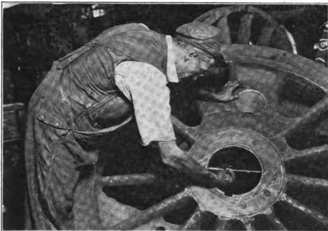
Fig. 4.—Calipering the Bore of a Wheel Center.
