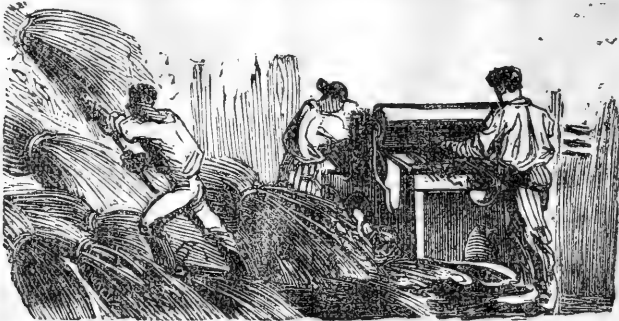
The above shows the breaking process by machinery. The first operator directs the stems by bunches to the rollers: the second receives the cleaned fibre and the third sends it towards the washing tubs, where the glutinous and woody matter is dissolved or disintegrated from the textile.
