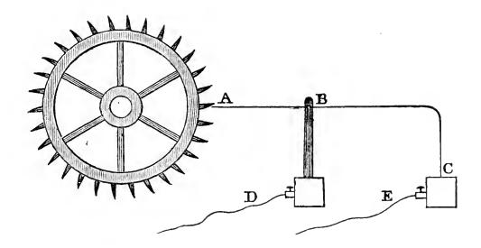
platinum bed, rest severally on a small block of wood. Each is connected by wires D and E, with a pole of the galvanic circuit, and the circuit is alternately broken and completed, by the rising and falling of the hammer. The latter operation takes about one tenth of a second of time.
