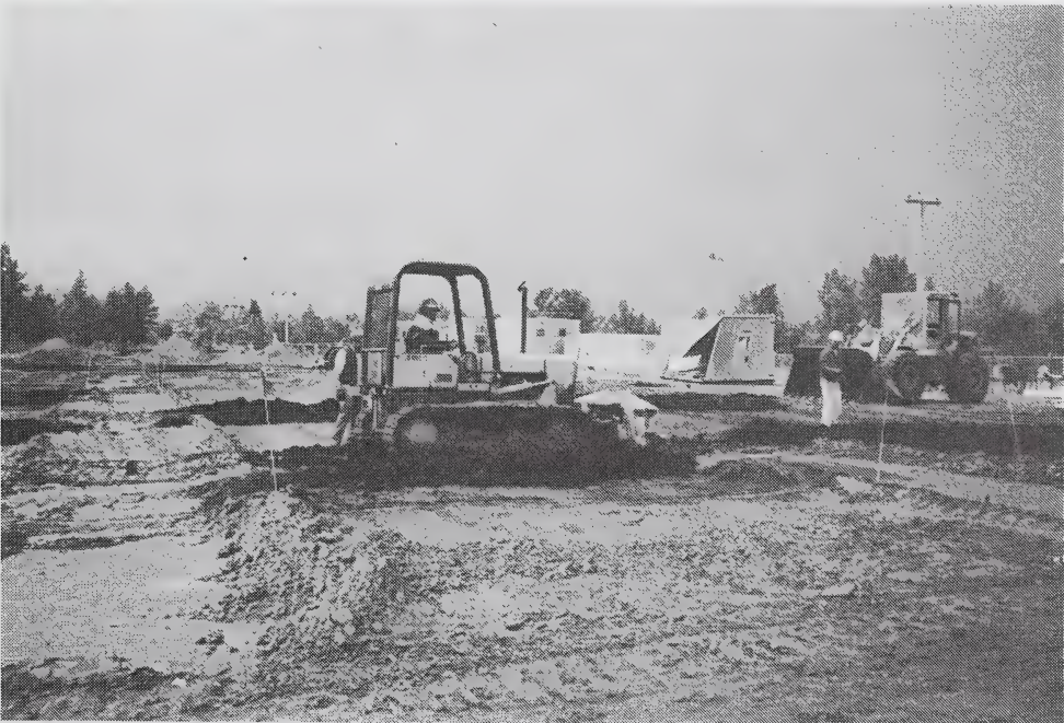
Figure 10. Application of manure using small bulldozer to 15 to 30 cm depth soil at Devon.
