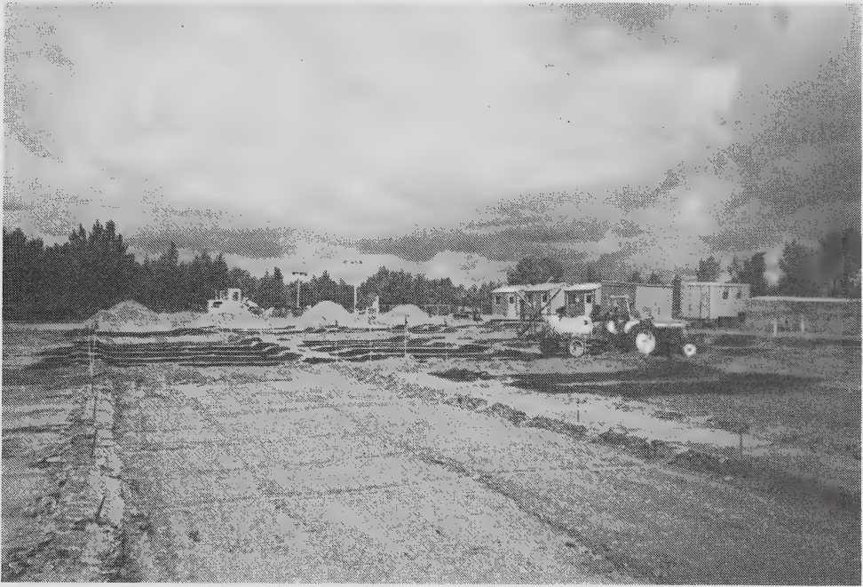
Figure 9. Application of activated charcoal with a tractor mounted spray unit to 15 to 30 cm soil depth at Devon.
