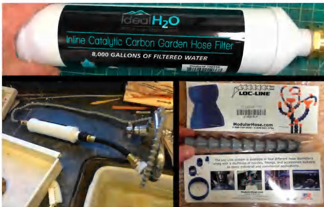
FIGURE 23. Water filtering system to reduce further contamination of the bones during rinsing, developed and installed by A. Davidson. Photographs by A. Davidson.
