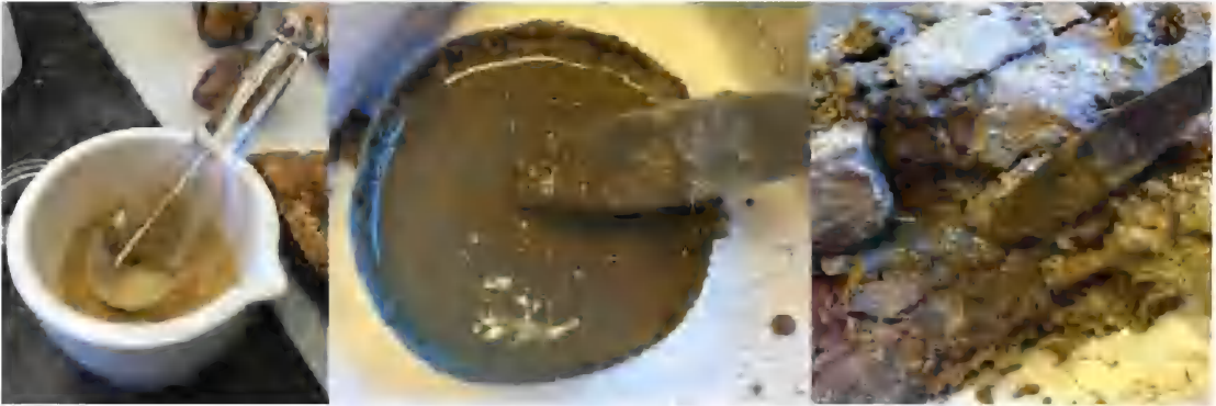
FIGURE 26. Mixture of pulverized sediment with highly diluted Paraloid B-72 (left) creates a strong gap filler for larger cracks (right), without adding extraneous filler material. It also remains soluble in acetone (center) and can be removed mechanically. Photographs by A. Davidson.
