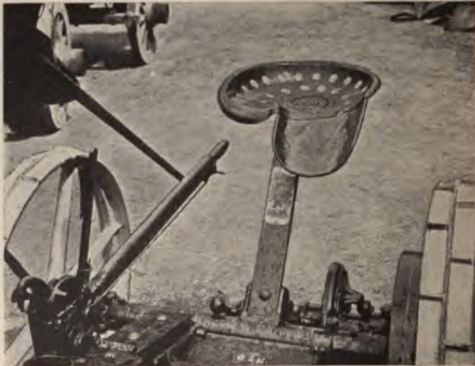
FIG. 25.—Seat of a mowing machine modified for a driver with a thigh amputation. ( Designed by M. Dor. )
