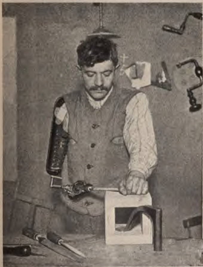
FIG. 13.—Carpenter using the Amar claw.
