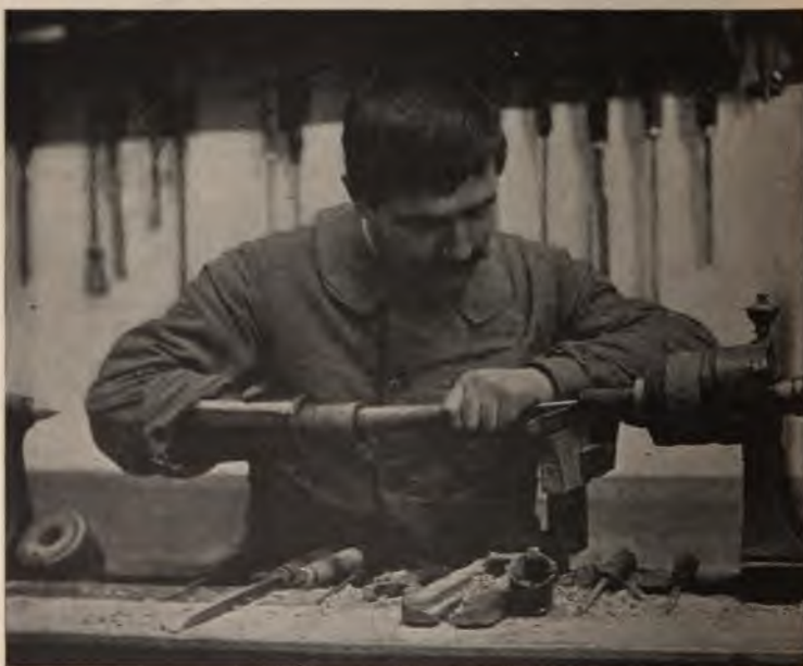
FIG. 23.—A French wood turner, Montpelier school, using simple tool holder.
