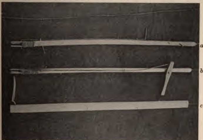
FIG. 24.—Adaptations of simple tools for one-armed worker: a , original form of weed puller; b , same modified for use of one-armed worker; c , trowel mounted to prevent stooping.
