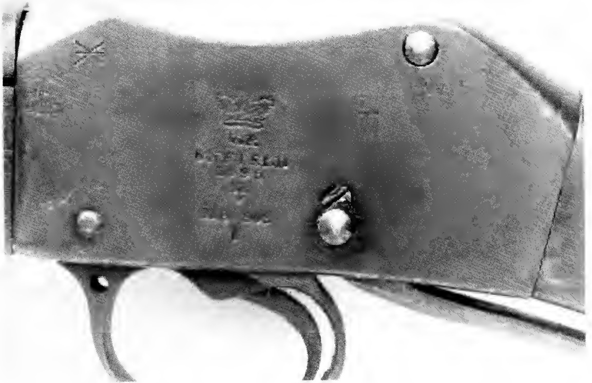
Figure 2 The Martini-Enfield Mark I conversion details found on the left side of the body. The royal cypher of Queen Victoria, the place and date of conversion, the steel batch mark and the Mark, in this case Martini-Enfield .303 inch Mark I. Note also the various proof and armourer's marks and the twin opposing broad arrows denoting sale or surplus. (Photo D. Elford, W.A.M.)
