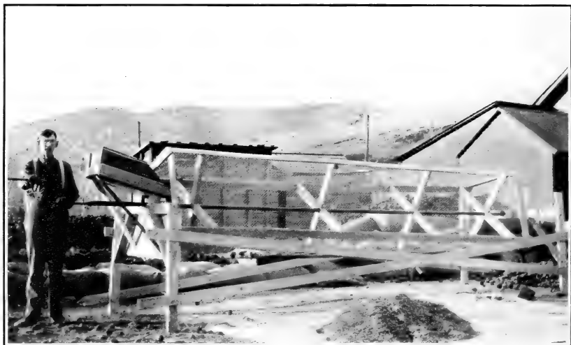
FIG. 2.—CHURN FOR REMOVING SEED FROM OPENED CONES.
