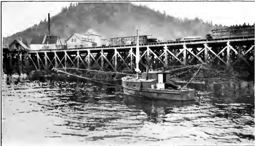
POWER BOAT USED FOR KING-SALMON TROLLING, SHOWING TWO OUT-RIGGERS TO WHICH LINES ARE ATTACHED. OTHER LINES ARE HANDLED FROM STERN OF BOAT.
