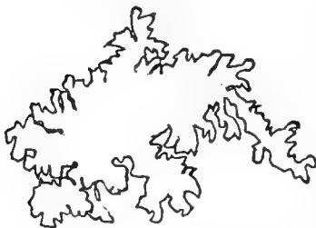
FIG. 3.—Metallic Iron in Sahara Sand, 100:1.
