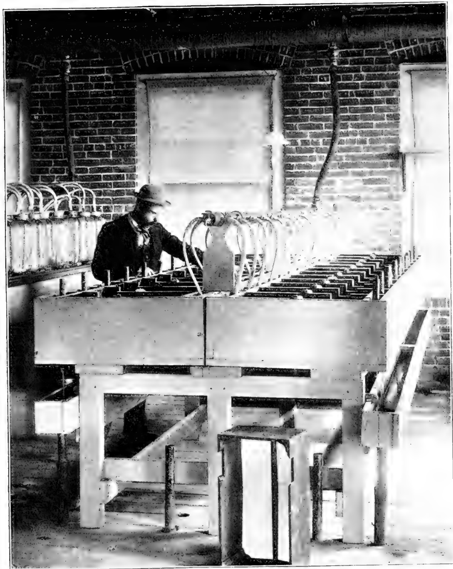
MCDONALD TIDAL BOXES, USED FOR HATCHING COD AND FLATFISH.
