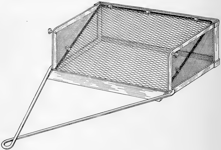
CUT 4.—Drill-dredge in position for work.
