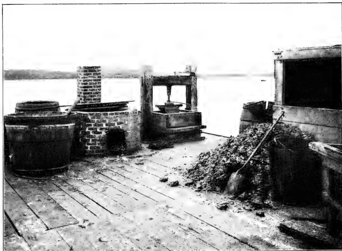
PRIMITIVE FORM OF KETTLE AND PRESS FOR RENDERING OIL FROM HERRING ON THE MAINE COAST.
