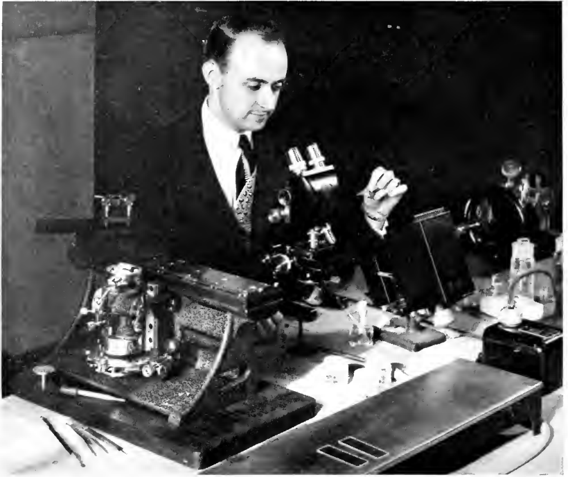
New research equipment includes a sliding microtome for cutting thin sections of plant material and a binocular research microscope with a low voltage light source. Donald Richards, Research Associate in Cryptogamic Botany, demonstrates their use.
