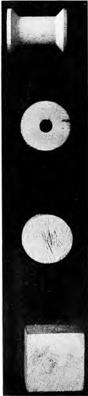
Steps in the manufacture of a one piece spool from Paper Birch
