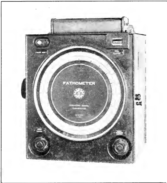
THE CONTROL PANEL OF THE FATHOMETER
