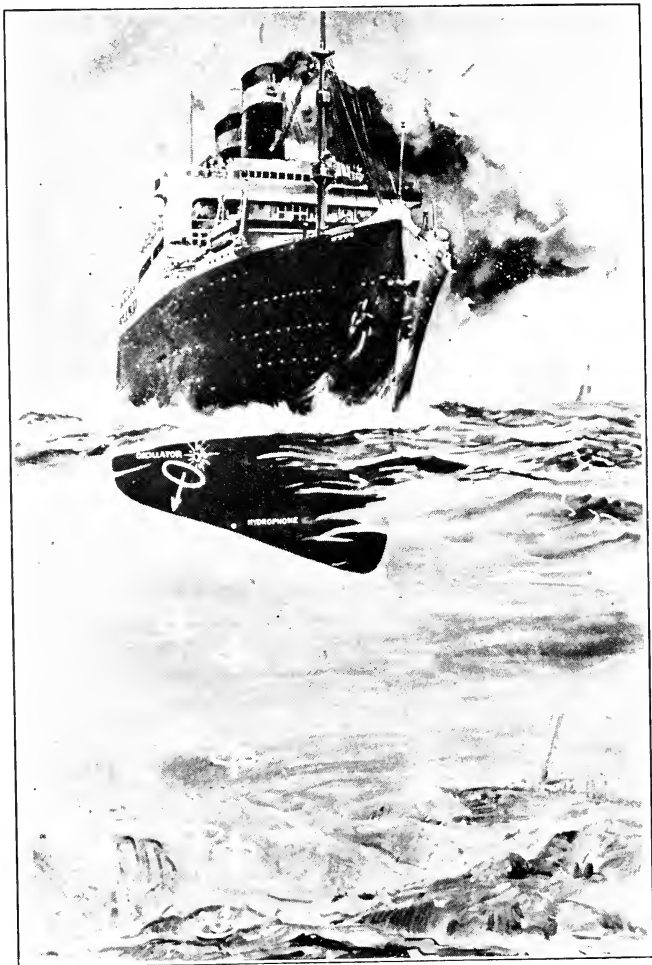
HOW A FATHOMETER MEASURES THE DEPTH
