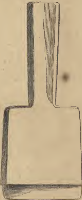
Simple form of handle with a blade with the same description of cutting edge.
