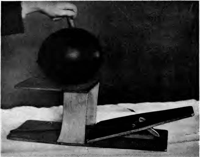
FIG. 13.—The balloon-gun for discharging balloons. A balloon is shown held in position on the platform just before the slamming-board is released by pulling the trigger. The base-board was 2 feet long.
