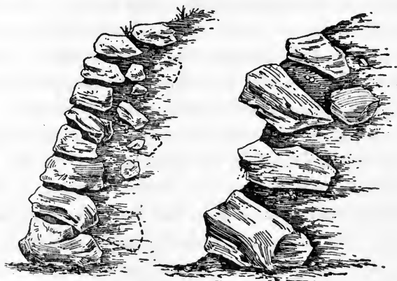
Building a Dry Wall. The wall should slope as shown in the first sketch. The second sketch illustrates a wrong method of building. Overhanging rocks should be avoided.
