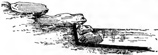
A Pool at the base of Rockery, the cement margin masked by rocks.
