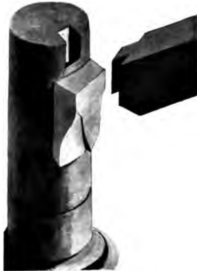
Fig. 52. Pillar with Corbel.
