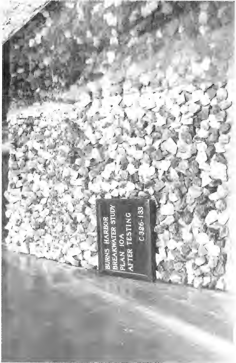
Photo 65. Lakeside view of Plan 10A after wave attack
