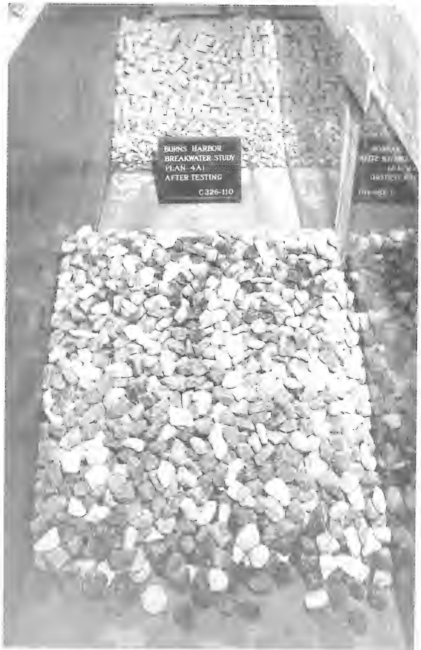
Photo 34. Lakeside view of Plan 4A1 after wave attack
