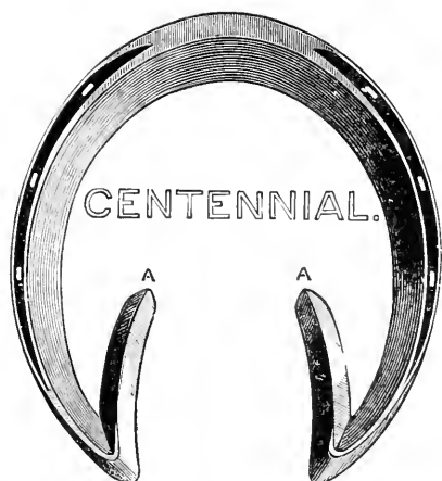
FIG. 117. ORIGINAL CENTENNIAL SHOE, DESIGNED BY S. T. HARRIS.
