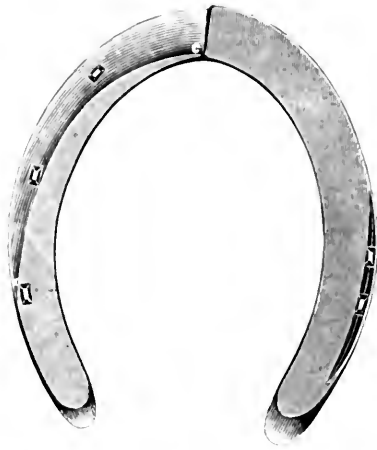
FIG. 104. RIGHT FRONT FOOT SHOE, TO PREVENT ANKLE, SHIN AND KNEE HITTING.
