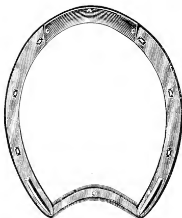
FIG. 155. FRONT FOOT BAR SCOOPED-TOE GRAB SHOE.
