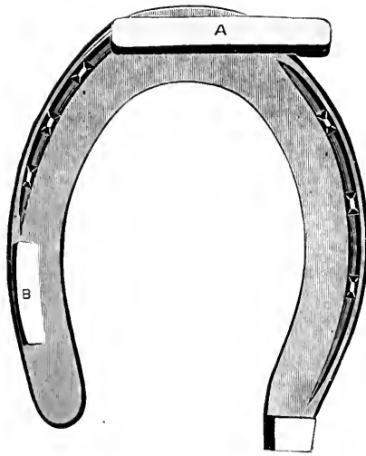
FIG. 175. SHOE TO PREVENT ANKLE HITTING. A, Projecting toe calkin. B, Side heel calkin.
