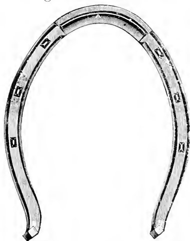
FIG. 197. HIND FOOT SHOE. WEIGHT, FOUR OUNCES.
