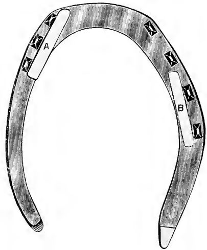
FIG. 174. SHOE TO CORRECT CUTTING INSIDE POINT OF TOE.
