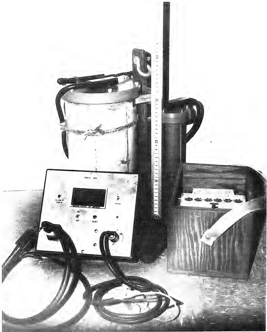
Figure B-4. Recording depth gage showing the sensing package, recording package and batteries for the recording package. The two cylindrical containers of the sensing package, which house the logic circuitry and pressure sensor, are mounted on a metal frame that is designed to maintain their proper attitude on the sea floor.
